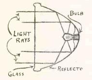
Fig. 2. How Headlight Focuses
