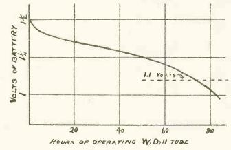
Fig. 1. How Dry Cell Lasts with WD Tube
