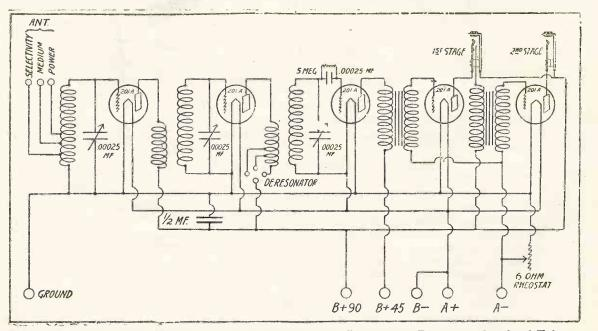
Fig. 3. Complete Wiring Diagram of Deresnadyne. Note Deresonator Between 2nd and 3rd Tube
