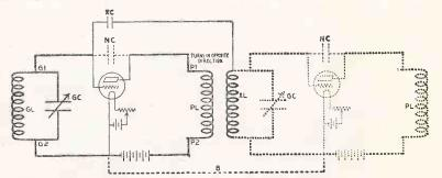
Fig. 1. Neutralizing Circuits of a Neutrodyne
