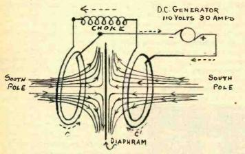
Fig. 3. How Coils Affect Diaphragm
