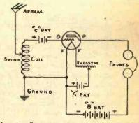
Fig. 1. Showing "A," "B" and "C" Batteries
