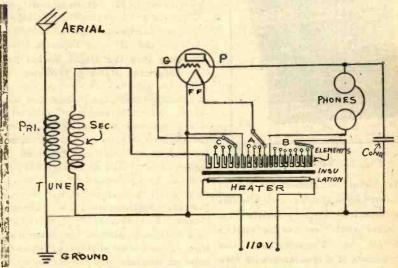
Fig. 6. Hook-up of Thermoformer
