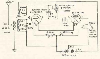
Radio Frequency Hook-up-No Transformer
