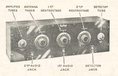
Fig. 2. Names of Neutrodyne Controls
