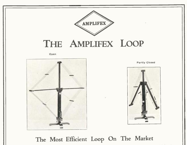
This is the Solenoid type of loop and collapses on the same principle as a Tripod by simply turning a thumb nut. The Amplifex Loop is wound with enamelled silk covered Litzendraht wire and has a very low resistance without any dead end losses as it can be tapped by a series of binding posts for either three hundred or six hundred meters. The full range of the Amplifex Loop is from 150 to 720 meters.
