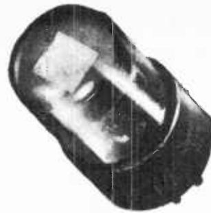
The FM tuning indicators shown here include the 6E5 and the 6AL7 tuning eye tubes along with a space-saving, side-indicating type tuning meter.
