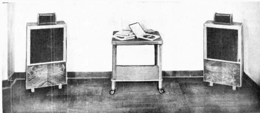
Fig. 10. Photograph of two speaker systems used to demonstrate two-channel sound.
