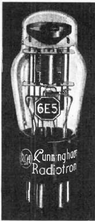
The FM tuning indicators shown here include the 6E5 and the 6AL7 tuning eye tubes along with a space-saving, side-indicating type tuning meter.
