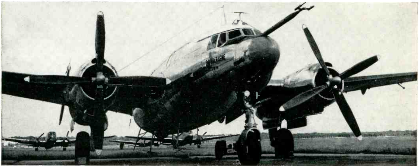
The French Air Force radar-testing "Bretagne" bomber was specially outfitted as an intercontinental TV relay station.
