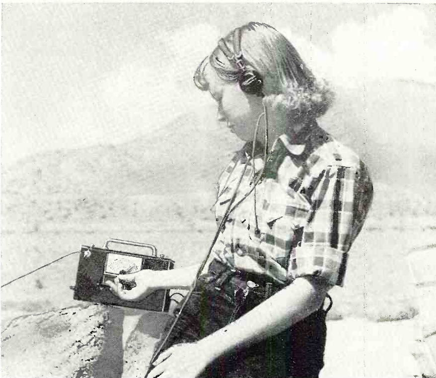
Fig. 2. Simple equipment can be built for Novice who likes to "rough-it." Power is gotten from car cigarette lighter socket.
