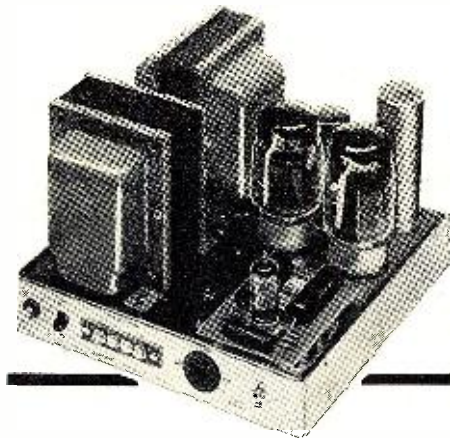
A wire cage over the tubes and a bottom plate are used to enclose the entire unit.
