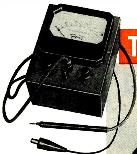
Fig. 1. Internal and external views of the completed transistor voltmeter.
