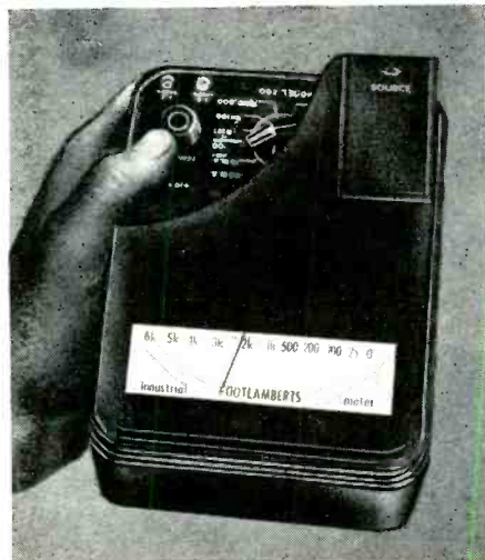
Fig. 4. Over-all view of adapter plugged into a Simpson Model 260 v.o.m. and in actual operation. Note the meter reading.
