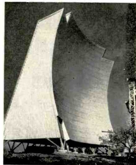
One of four 60-foot "big screen" Blaw-Knox antennas used in new microwave scatter link.
