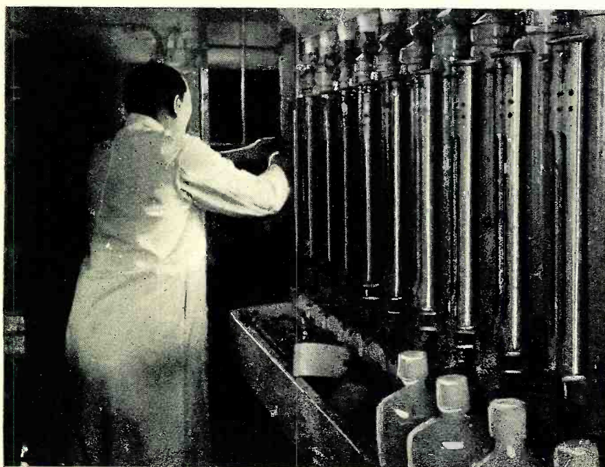
Scientist puts finishing touches on some of the lab equipment before a cruise. Objects in rack at right are Nansen bottles with deep-sea thermometer frames, used for capturing water samples at different depths. From Nansen bottles samples are transferred to glass or plastic storage bottles which are shown at lower right.
