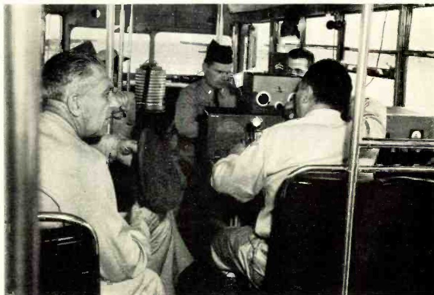
Civil Air Patrol communicators operate a high-frequency rig installed in a surplus Air Force bus which has been converted into a combination mobile communications station and a mobile operations headquarters for directing rescue work.
