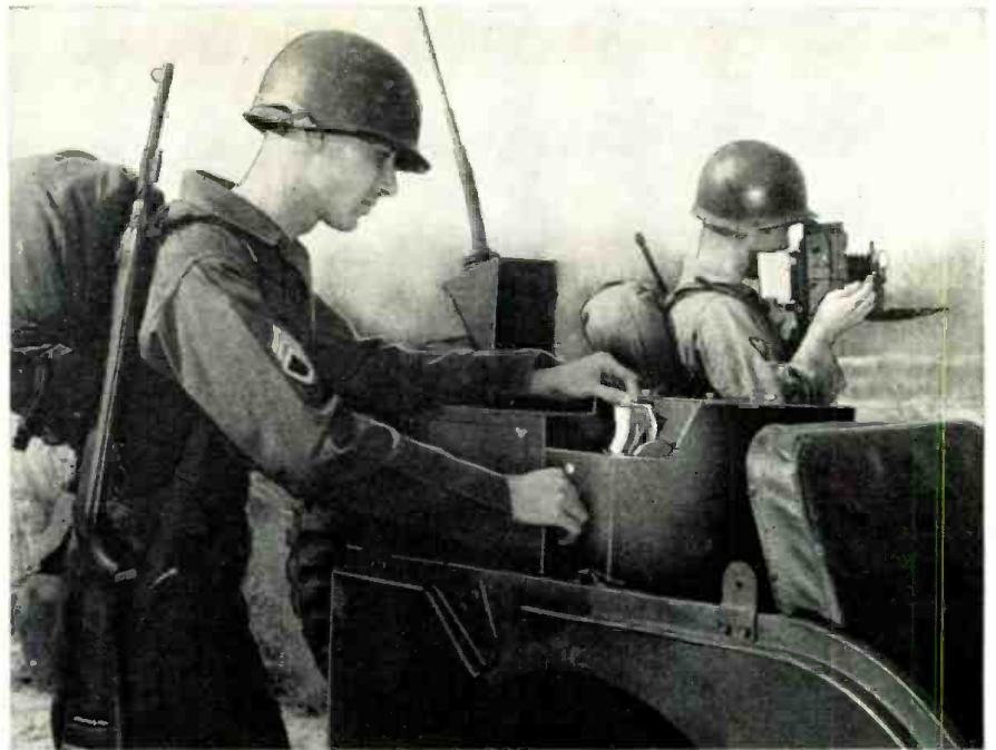
Operation of the new Signal Corps field facsimile set through jeep-mounted gear.
