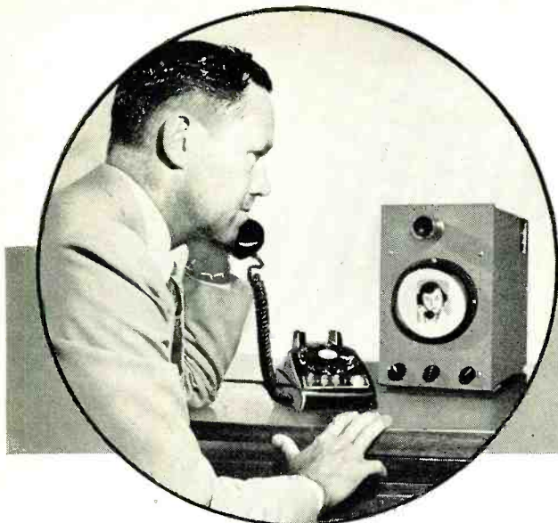
W. E. Kock of Bell Telephone Laboratories shows how one experimental model of a Picture-phone would be used. Protruding above the picture screen is the camera lens. The knobs below the screen are for turning on the set and for defining the picture.
