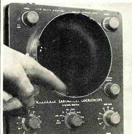
The re-inforced screen in place on scope.
