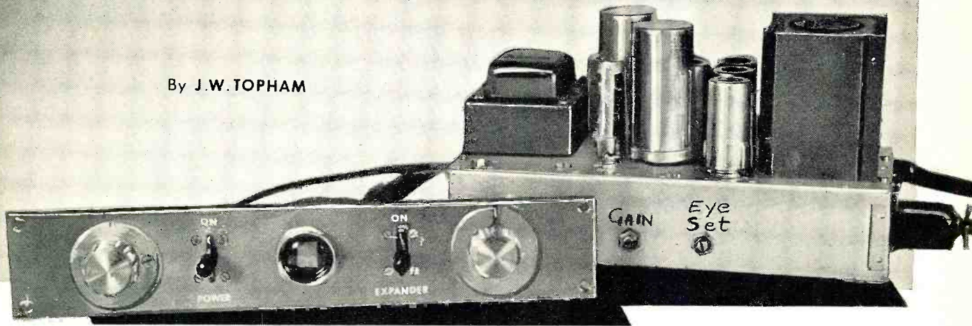
Fig. 1. Over-all view of remote control panel (left) and chassis housing expander and power supply (right). Controls on the panel are from left to right: master gain of complete system, power switch, eye tube, expansion switch, and the expansion set control. See diagram, Fig. 2.
