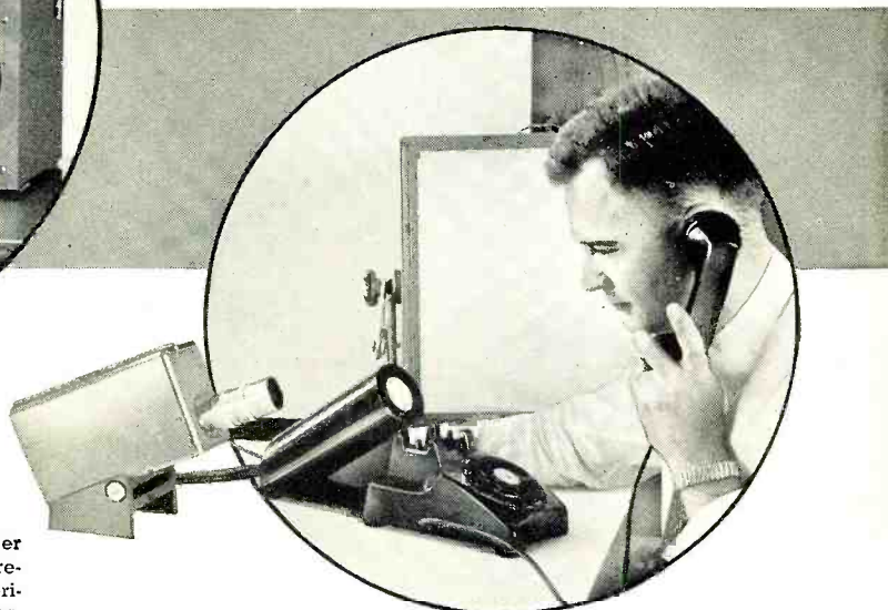
W. E. Kock of Bell Telephone Laboratories shows how one experimental model of a Picture-phone would be used. Protruding above the picture screen is the camera lens. The knobs below the screen are for turning on the set and for defining the picture.
