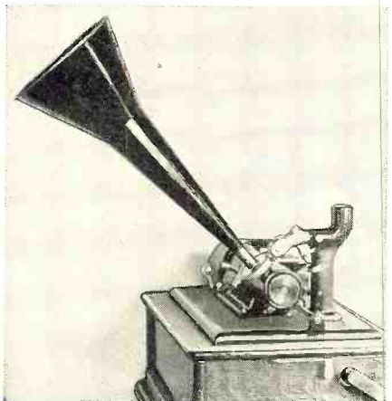
Fig. 16. Recording attachment included a horn, recorder, and a special basket.
