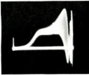
Fig. 4. The response of the Q demodulator (a typical low-frequency chroma circuit) can be obtained with this arrangement. However, as shown at left, the rectification and filtering of the PEAK-
