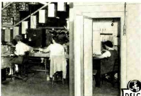
In the audio test booth, the speaker is checked for its ability to deliver good listening. In the background you can see a small section of the speaker production line.
