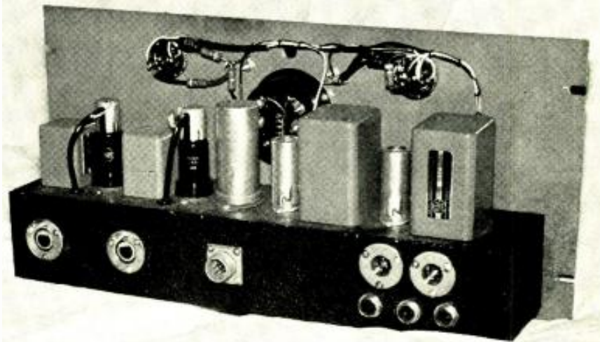
Rear view of unit. Note particularly the type of jacks and plugs that were used in the construction of this unit. It is important that all of these components be of the shielded type to prevent hum pickup. The jacks and plugs are, from left to right: Mic. 1, Mic. 2, power cable connector. (far right, top) 50 and 500 ohm outputs, (far right, bottom) Phono 1, Phono 2, and tape playback inputs.
