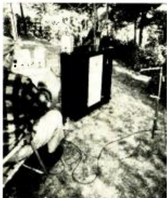
COVER PHOTO: Free-field response measurements being made on the "Fold-a-flex 12" described in this issue. The E-V 655 and Shure 98-99 calibrated microphones connect to a Heath AV-2 a.c. vacuum-tube voltmeter. (Ektachrome by Jay Seymour)
