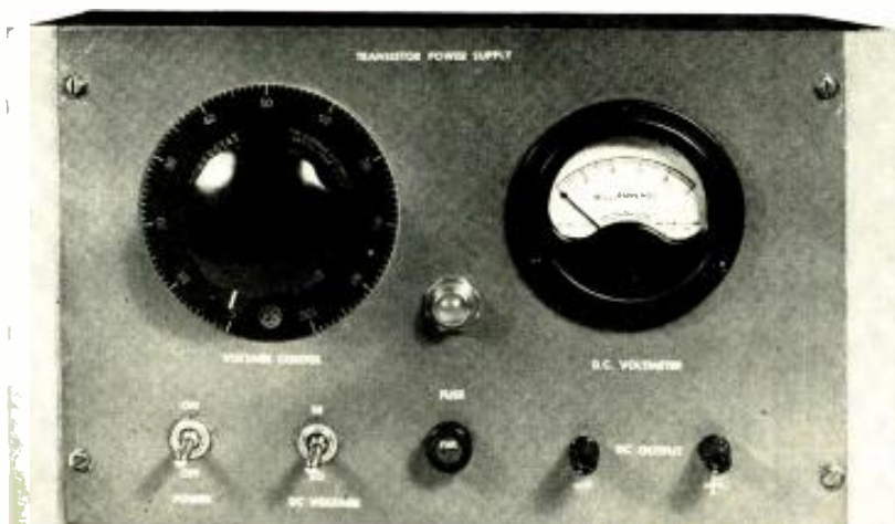
Fig. 1. Front panel view of the power supply unit. An optional meter for reading current can be added.
