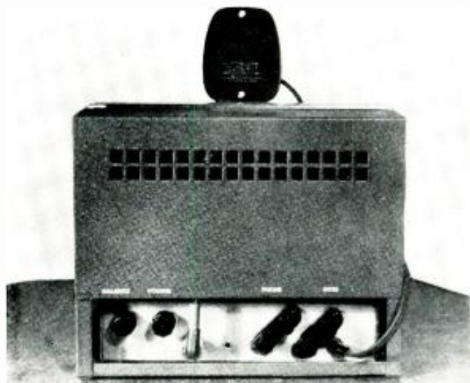
Fig. 4. Rear view of cabinet showing potentiometers R_1 and R_2 , the microphone connector, J_1 , and the two sets of terminals.
