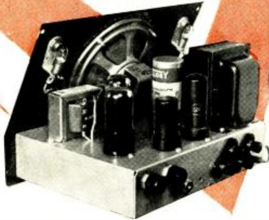
Fig. 1. Front and rear chassis views of the switchless intercom. The entire unit is housed in an 8" x 10" x 8" sloping panel cabinet.
