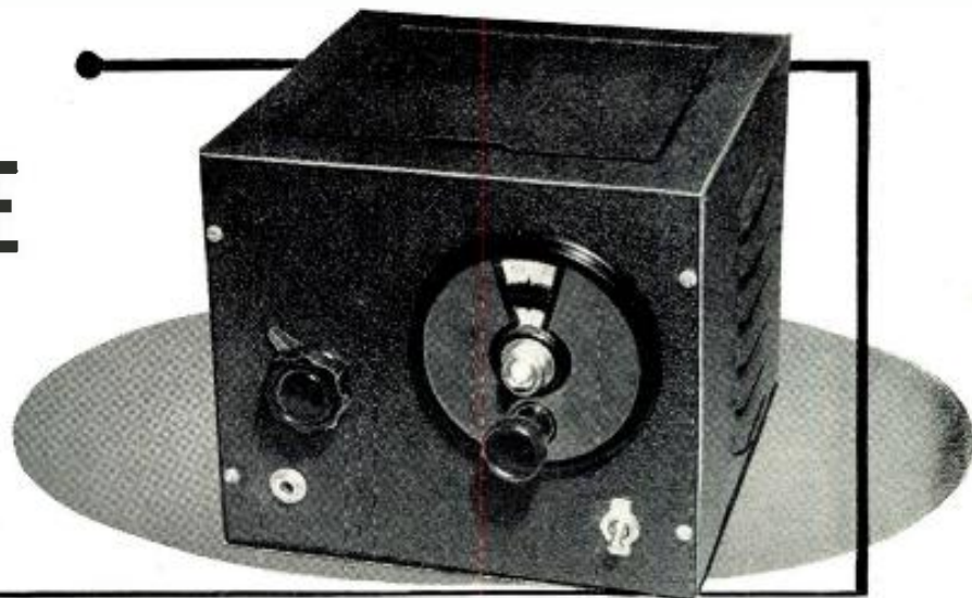
The regeneration control (knob at left) is a 140- \mu fd. variable condenser, providing smoother regeneration than other methods. Receiver is housed in an 8"x8"x7" cabinet.
