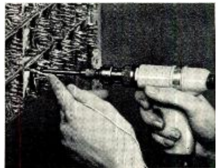
Power tool whips wire on terminal in fraction of a second. There is no heat which could damage miniature components . . . no dropped solder or wire clippings to cause trouble later.
