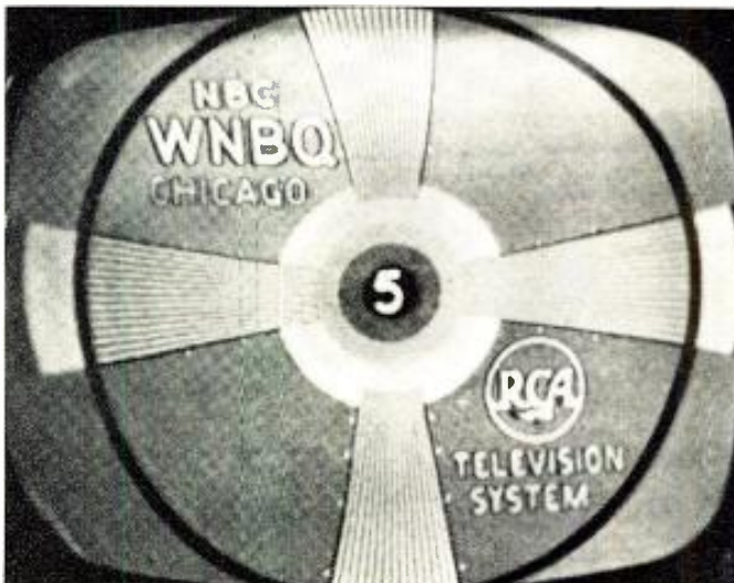
Fig. 3. Picture obtained after a booster was installed.
