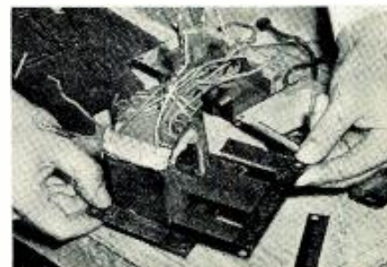
Fig. 2. How transformer core is disassembled.
