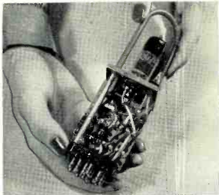
Close-up view of plug-in turret used in the OARAC electronic calculator.
