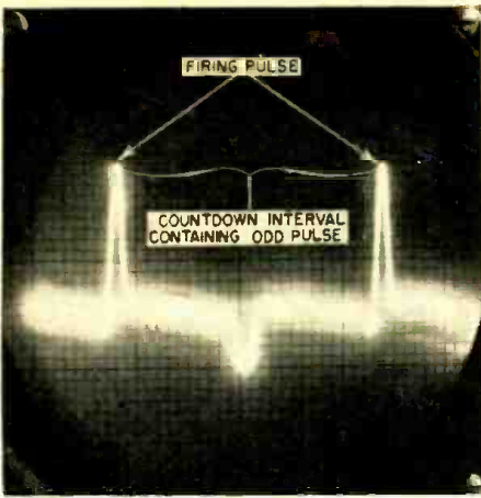
Fig. 7. "Divided by 2" counter pulses on scope when connected to "Test Plug \div 2 ." Every second pulse triggers \div 2 oscillator.
