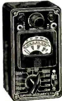
Model 770 is an accurate pocket-size V.O.M. Measures only 3/16" x 5/16" x 2 1/4".
