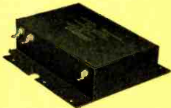
This power line filter provides correct output voltages from sources of 50 to 400 cycles ... noise attenuation is from 14 KC to 400 MC ... 29 cubic inches.
