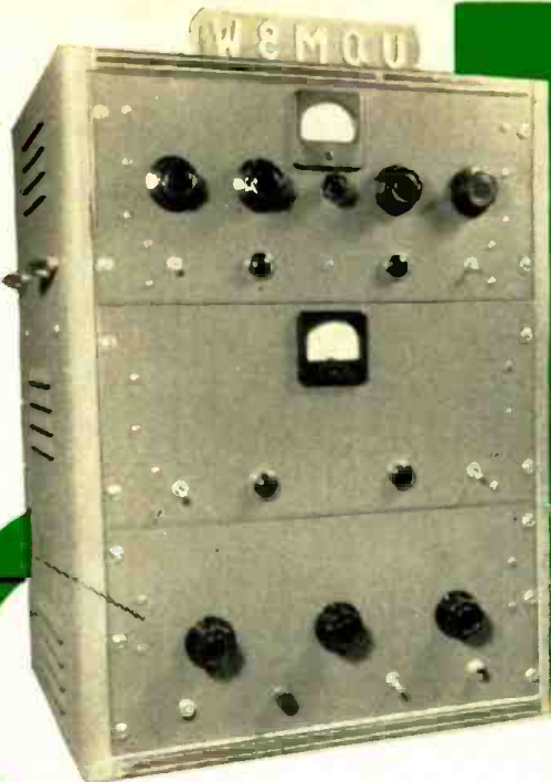
The r.f. section of the author's 250-watt transmitter was described in RADIO & TELEVISION NEWS for June, 1952. The modulator occupies the center section of the rack. The speech amplifier is below.
