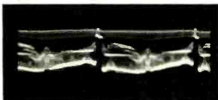
Fig. 1. Signal from plate of video amplifier fed to a.g.c. tube control grid.
