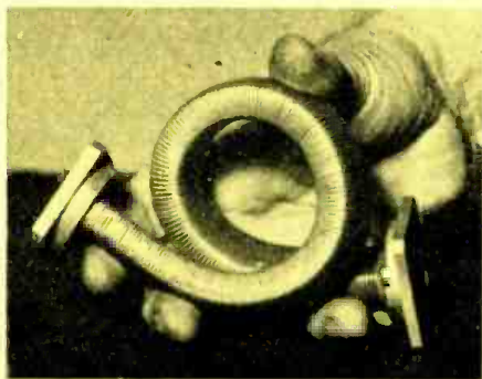
Fig. 3. A demonstration of the flexibility of flexible rectangular wave guide manufactured by Flexible Hose Mfg. Co.
