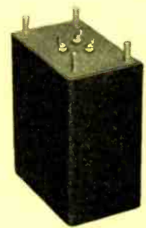
This band pass filter is designed for sharp cut-off at both ends of the range ... 10,000 ohms ... case dimensions 1¾" x 2½" x 3¼".
