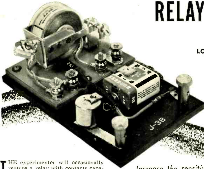
Fig. 1. Transistor setup for increasing relay sensitivity. Author's unit was built on Bakelite strip but may be housed in a standard Bud "Minibox" if desired.
