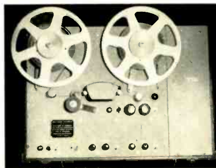
The multi-channel "reproduce" tape transport unit of the new system.
