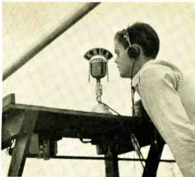
Single-channel remote b.c. amplifier shown mounted under table at ball park. Power supply and amplifier are spaced at least 1½ feet apart to reduce hum pickup.
