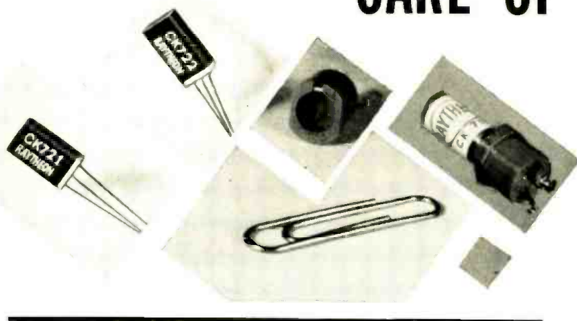
Fig. 1. The CK721 and CK722 junction-type transistors. To the right is shown the CK716 in its specially-designed molded socket housing.
