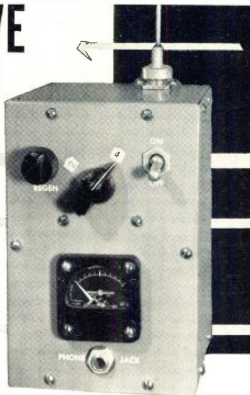
Fig. 1. Front panel view of the compact, home-built superregenerative field strength meter.
