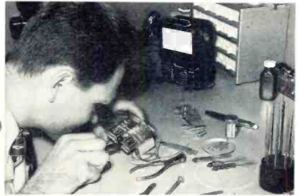
Using a jeweler's tool and magnifying glass, this Ryan electronics engineer wires a packaged subminiature circuit used in the radar equipment developed by Ryan.
