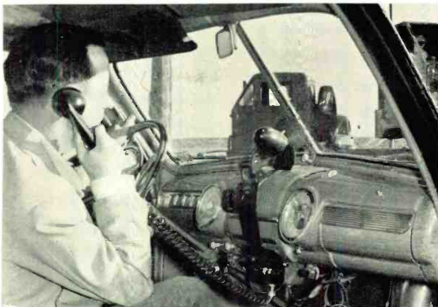
Foreman W. J. Lynch of the Colorado Interstate Gas Company uses his General Electric two-way radio equipment to talk to the company's headquarters 15 miles away.
