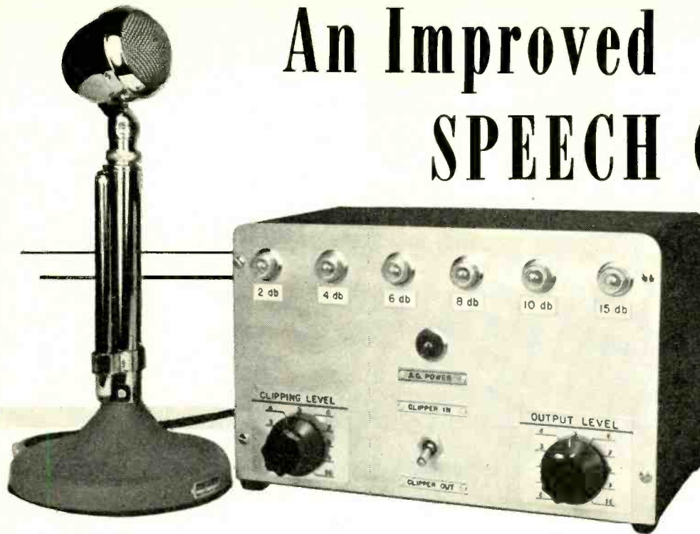
Fig. 1. Front panel view of clipper. The unit indicates clipping level directly in decibels by means of flashing neon lamps.
