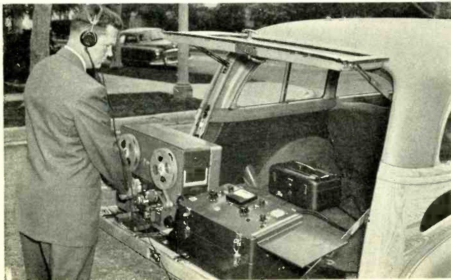
Fig. 2. The portable RCA sound recording system shown in use on movie location.
