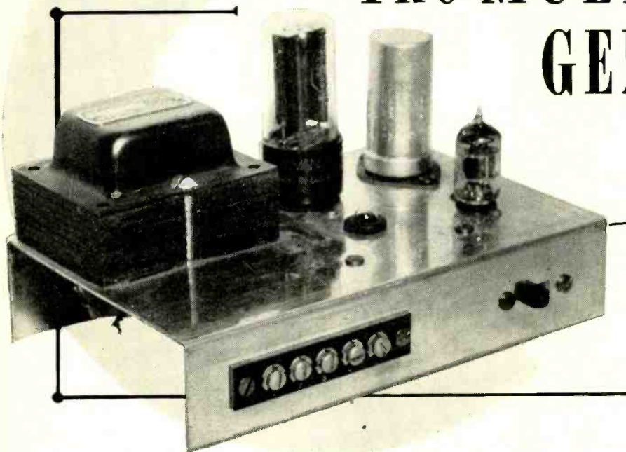
Fig. 1. Over-all view of the "Multi-Signal Generator." The entire unit measures 7\frac{1}{2} " x 5" but provides 60-cycle sine-wave, saw-tooth, and square-wave signals.
