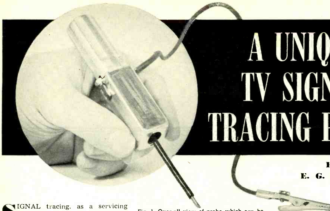
Fig. 1. Over-all view of probe which can be used with both medium and high-gain scopes.
