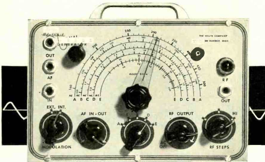
Fig. 1. Three units must be added to the panel of your signal generator if it is to be used as a grid-dip oscillator. Jack J_1 , labeled "Probe," is in the upper left-hand corner. S_1 , the link switch, is just below and to the right of J_1 . C , depending on the type of indicator used, mounts on the right side of the panel above and to the left of the pilot light.
