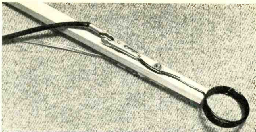
Fig. 3. Over-all view of probe coil. The unit consists of 6 turns of No. 14 enamel wire, 1\frac{3}{8} " in diameter. After the turns are cemented together, the coil is cemented to the end of a wooden handle. The leads are fastened to soldering lugs mounted on the handle by means of 6-32 machine screws. Alligator clips on signal generator's output test lead attach to the lugs and energize the coil with r.f.
