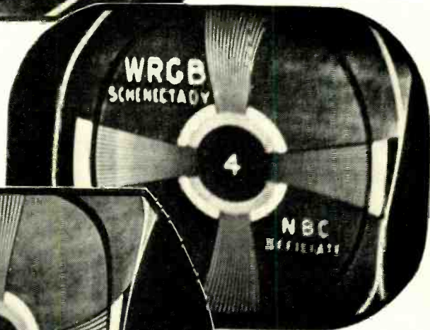
Fig. 8. Another example of hum in the picture tube. Replace the tube first before checking the power supplies.
