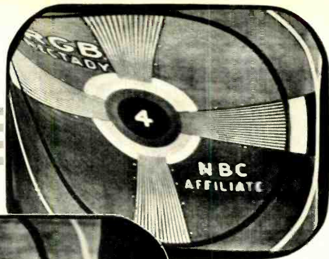
Fig. 5. If a metal-cone picture tube has been magnetized, a condition such as shown here results. The tube must be demagnetized. See text for instructions.
