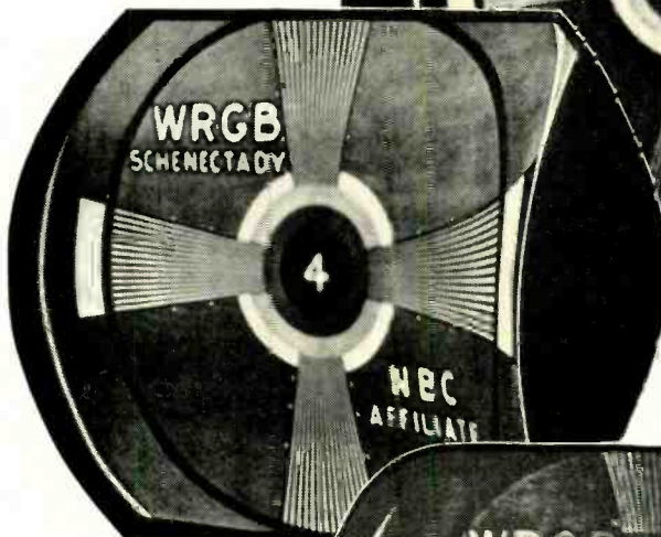
Fig. 8. Another example of hum in the picture tube. Replace the tube first before checking the power supplies.
