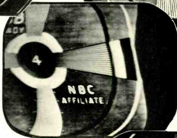
Fig. 7. Hum in picture causes curved or distorted raster edges as shown here and in Fig. 8. Try replacing the TV picture tube.
