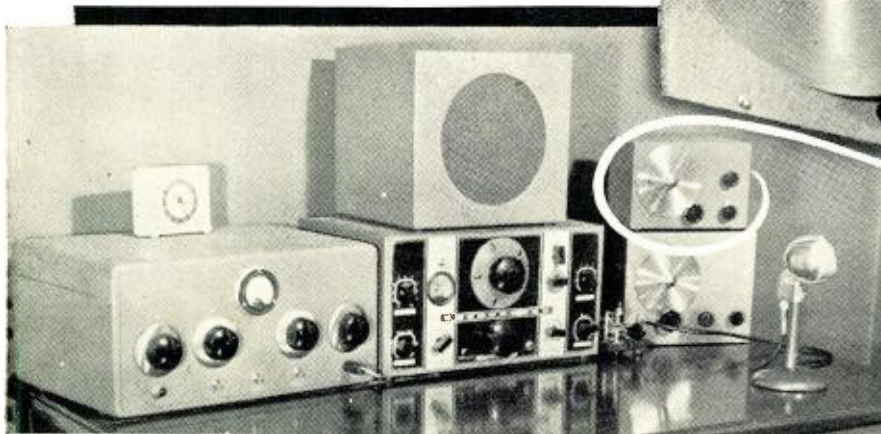
Author's operating desk. An NC-100X receiver is flanked by a 150-watt amplifier and two exciters (one covering ten meters and the other the 3-band unit described). A single sideband adaptor is also used with this equipment on 75 and 20 meters.
