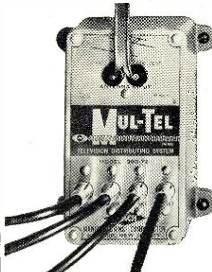
Fig. 1. Over-all view of the "Mul-Tel" unit which is designed to provide multiple outlets for single family dwellings. The box is placed out of sight near the antenna.
