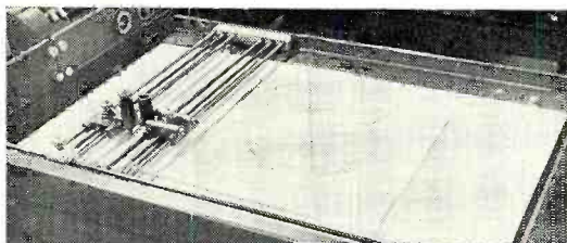
Electronic analog simulating equipment. This is part of the one-hundred amplifier installation and demonstrates the solution of a simple beam problem. Equipment was built at University.
