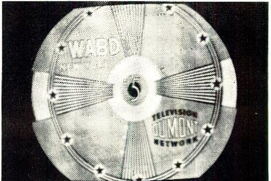
Fig. 4. Pattern on the cathode-ray screen after ignition noise has been eliminated. Notice how the black streaks which were visible in the pattern of Fig. 1 have now been eliminated and how the over-all picture contrast has been considerably improved.
