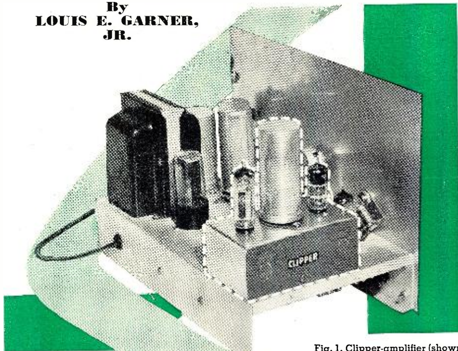
Fig. 1. Clipper-amplifier (shown dotted) mounted on chassis of "Deluxe Pulse Generator" unit.
