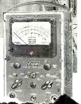
Mr. Al Goldberg, Assistant Chief Engineer of CBS-Columbia, and Harry R. Ashley, President of EICO, inspecting the use of the EICO Model 221 Vacuum Tube Voltmeter and Model HVP-1 High Voltage Probe at the Sweep Frequency Troubleshooting Position on the CBS-Columbia Color Television production lines.
