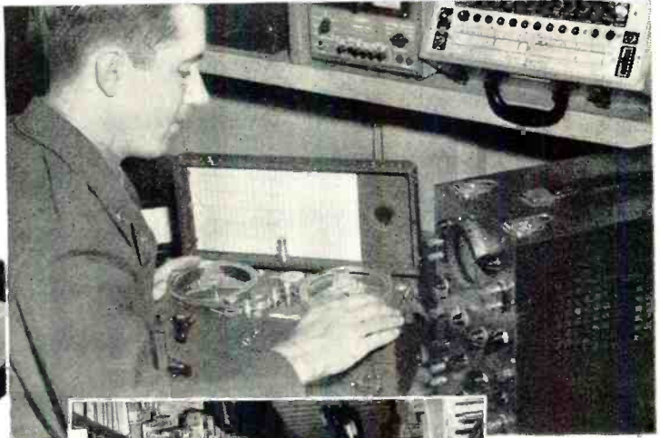
Checking a Stancil-Hoffman "Minitape" machine is function of maintenance section.
