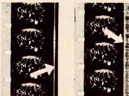
Fig. 1. (Left) Variable area sound track, and (Right) the variable density sound track.
