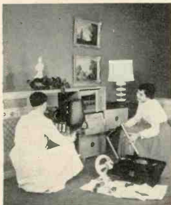
COVER PHOTO: Making final adjustments on a custom installation. Housed in Jensen "Customode" cabinets are Jensen speaker, Radio Craftsman 16" TV set and AM-FM radio, and Talk-A-Phone "Chief" intercom with handset. A Milwaukee Stamping record changer is housed in bottom drawer. (Kodachrome by Art Haug)
