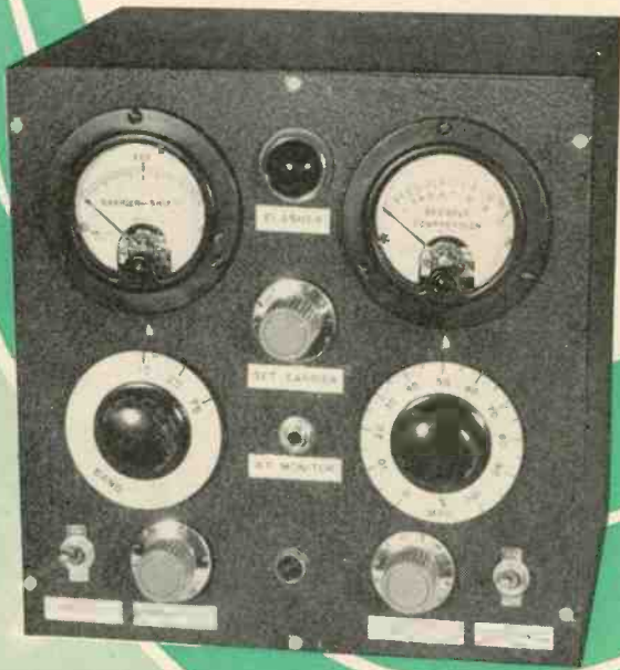
Fig. 1. Front view of unit. Modulation peak percentages up to 100% can be measured.
