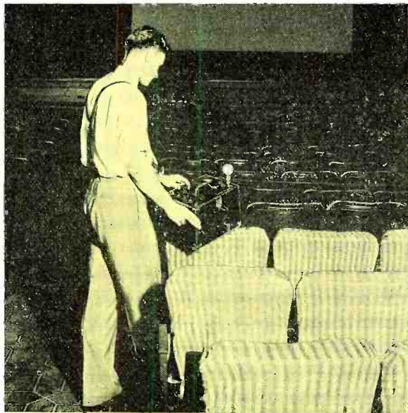
The General Radio type 759-B sound level meter being used to perform acoustic measurements in a motion picture theater.
