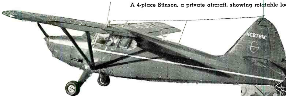
A 4-place Stinson, a private aircraft, showing rotatable loop antenna.
