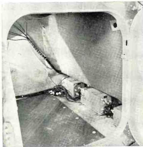
The v.h.f. transmitting and receiving equipment installed in a Beach Bonanza baggage compartment.
