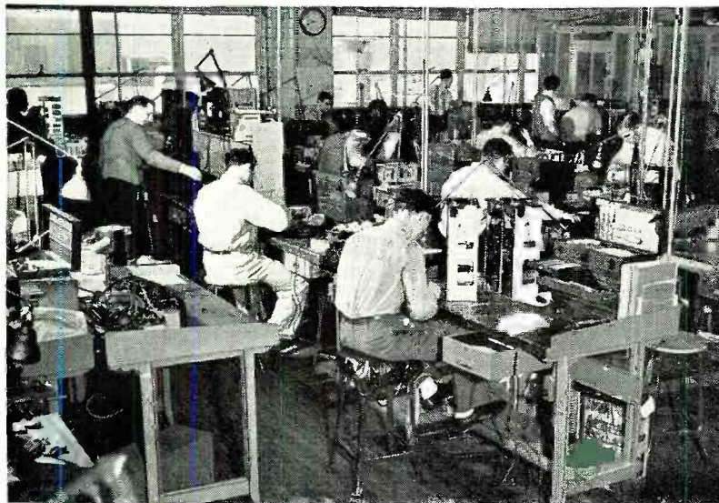
An over-all view of American Airlines' radio overhaul shop. As mentioned in the article, the large commercial outfits stress preventive maintenance and subject all radio equipment to periodic and thorough checks.
