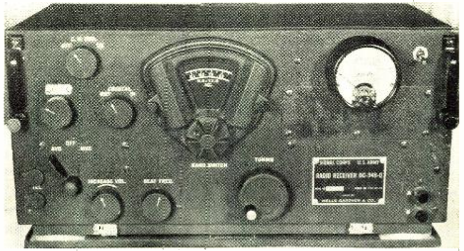
Fig. 2. Front panel view of the BC-348-Q on which the "S" meter was mounted. The panel projection type meter was used in order to avoid a large hole-drilling job.
