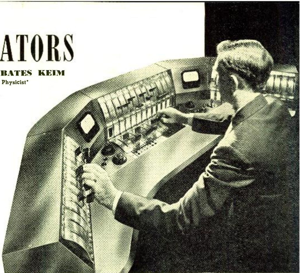
Fig. 1. The Roxy Theatre Control Console. Provision is made for 52 slide attenuators; 38 are shown in operation. In left foreground, front rotary attenuator is stereophonic control
