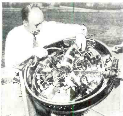
Top view of transmitter-receiver. Gyroscope and motors keep unit approximately level during flight.
