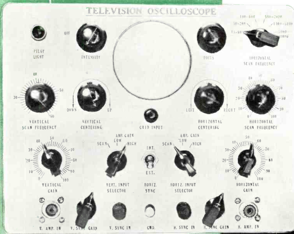
Front panel layout of completed television oscilloscope shows position and identity of all operating controls.
