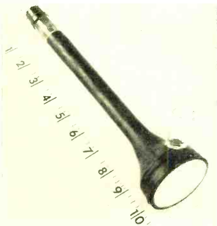
Fig. 4. The new 2½ inch magnetic cathode-ray tube, type 3NP4. Picture size is 1.4 inches by 1.86 inches.
