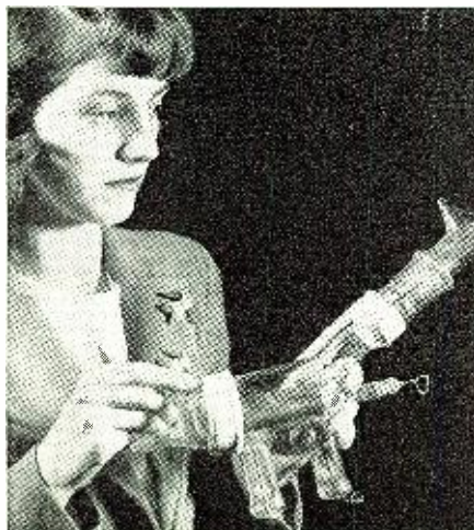
Fig. 7. The "Giraffe"—an electronic tube used in conjunction with a Geiger counter is shown at the Westinghouse Laboratories.
