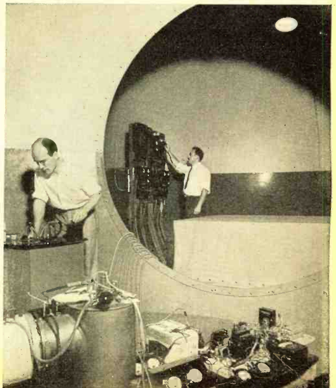
Fig. 5. Inside the spherical terminals of the Van de Graaff Generator installed at Massachusetts Institute of Technology.
