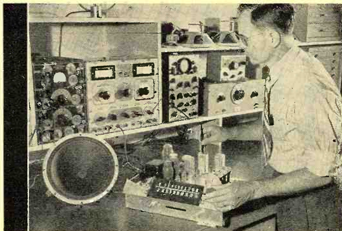
Equipment engineer checking preliminary alignment of radio. Several methods are tried, but the simplest and most foolproof technique is adopted for inclusion in the service note. Voltage data on the set is also taken at this time.
