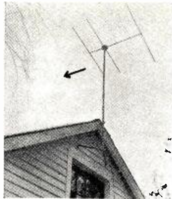
Fig. 8. High-gain, ghost-free reception is obtained with a single channel antenna, consisting of director, dipole, and reflector.
