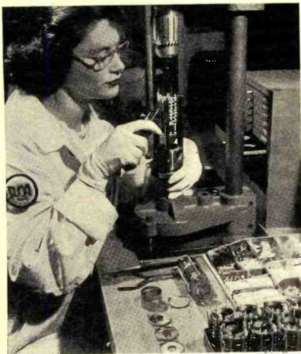
8 A non-reflecting carbon coating, designed to keep stray electrons from the picture screen, is next applied with a long-handled brush.
