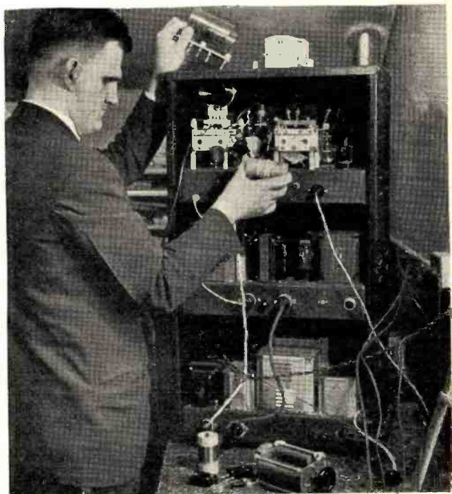
A fine example of the excellent workmanship seen at the school is the instructor's pet transmitter. The rig was built entirely by Mr. Gunderson, including drilling of chassis and panels.
