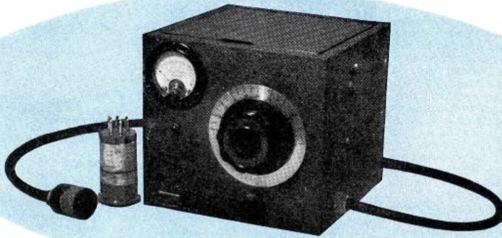
Panel view of completed instrument. A metal cabinet measuring 7" x 7" x 7" was used.
