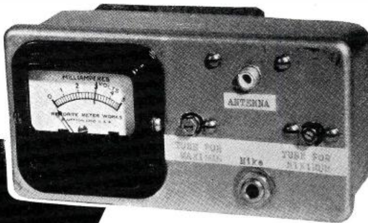
Front panel view of completed instrument. Note that meter has a 5 ma. movement. This is used when a 45-90 volt "B" supply is available. If a 22½ volt supply is used then the meter should be a 0-1 milliammeter movement.
