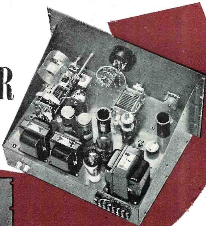
Two views of the completed unit. Although home constructed its appearance compares favorably with many commercial transmitters.
