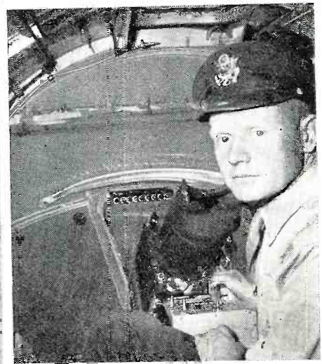
★ Col. H. T. Ailness, in command of remote control B-17 operations for the coming atom bomb test, is shown in nose of the "Mother" ship with television scope and control box with which "Drone" B-17 can be flown at a distance of 150 miles from "Mother" plane.
