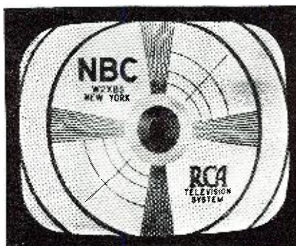
Fig. 1. Advancing the contrast control too far produces results similar to this.
