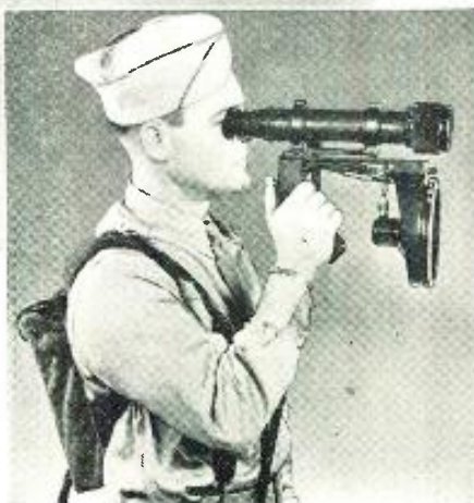
Top photograph shows the sniperscope as it appears in conjunction with the .30 caliber carbine. Mounted on the carbine, this unit permits the sniper to locate the enemy and then fire. The snooperscope shown at the right is used for signalling and as a detection device. Fire control officers used this unit to direct the battery barrages.
