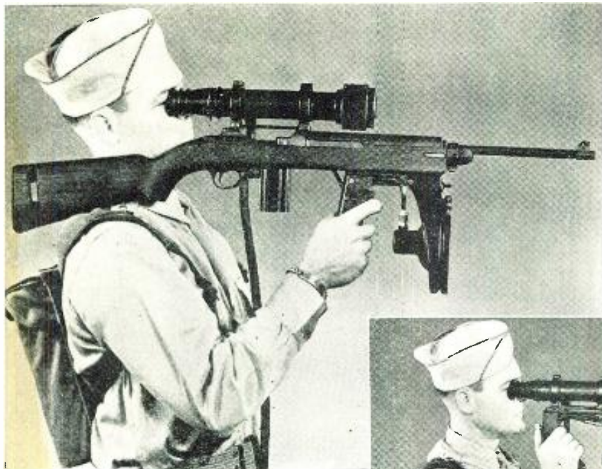
Top photograph shows the sniperscope as it appears in conjunction with the .30 caliber carbine. Mounted on the carbine, this unit permits the sniper to locate the enemy and then fire. The snooperscope shown at the right is used for signalling and as a detection device. Fire control officers used this unit to direct the battery barrages.
