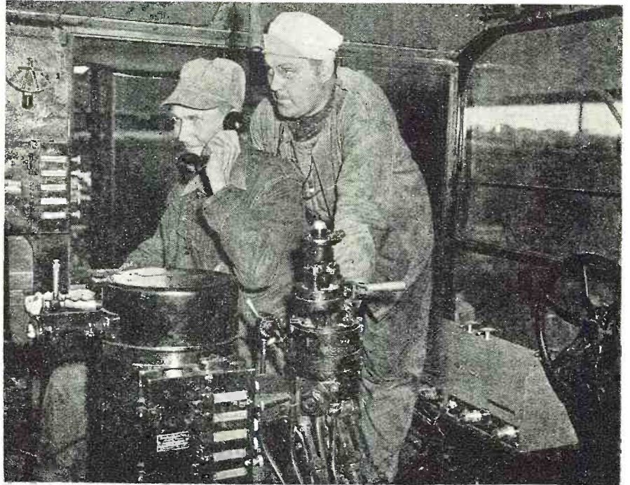
Engineer of one of the Rock Island Lines' 5400 series freight diesels gets his "go ahead" or "hi-ball" orders by means of two-way FM radio.
