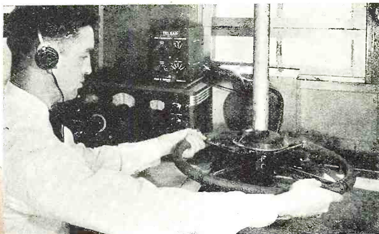
Adcock direction-finder—so critical in balance that a spiderweb across the transmission line will upset calibration. Operator is K. W. Miller, W5AOC, Asst. Supv.
