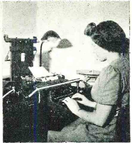
Transcribing copy from Boehme tape. Operator controls speed by foot.
