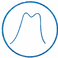
Good response curve of superheterodyne, having flat-top i.f.'s.
