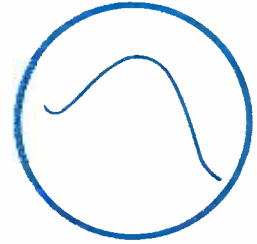
Improperly aligned tuned circuit, giving adjacent channel interference.
