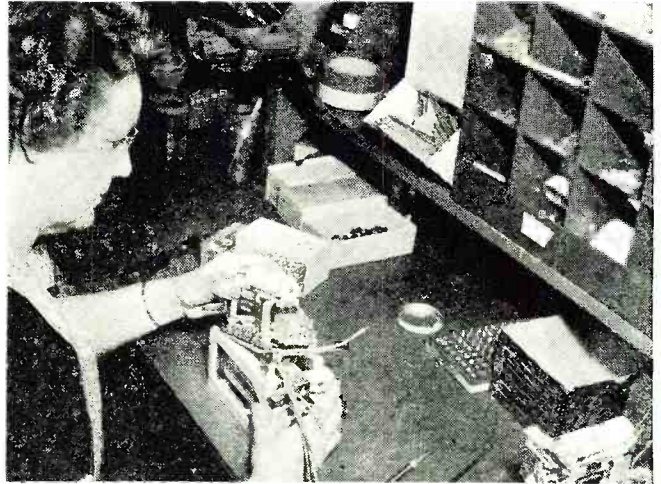
Keying relay and capacitors being placed on antenna-tuning coil, making a complete sub-assembly.
