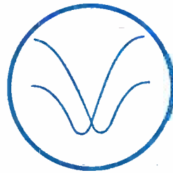
Crossover point not at center, showing that detuning of secondary exists.
