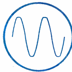
Overload distortion with cut-off flat peaks. Gain control turned too far up or improper grid bias.
