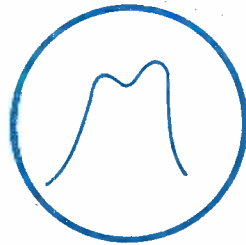
Circuit requires slight adjustment of the trimmers to bring it to symmetry.
