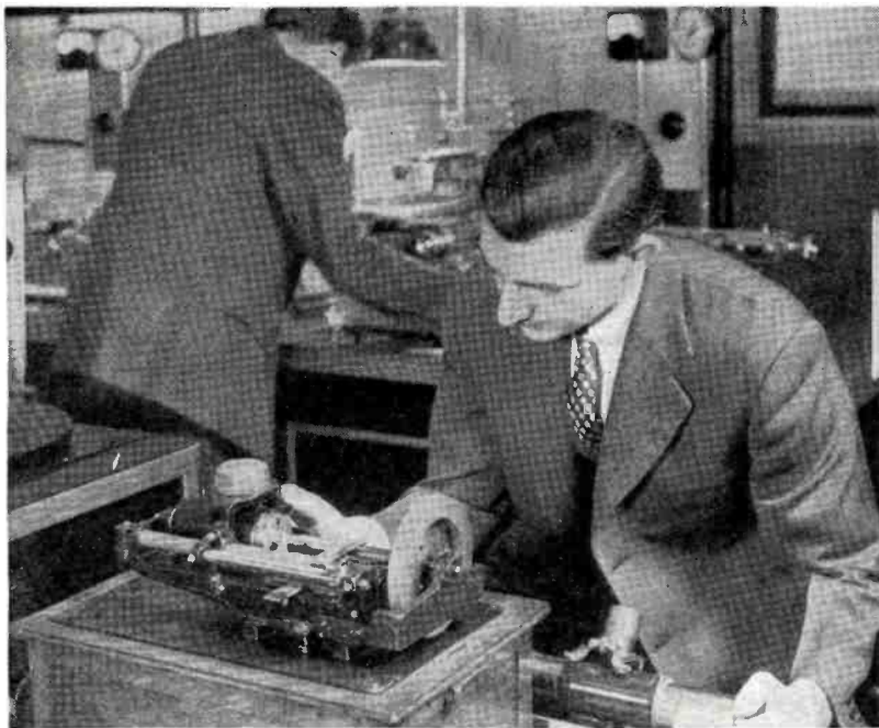
Dr. Arthur D. Semmig operating oldtime cylinder transcribing machine. Crystal pickup output is fed to Scully recorder for dubbing.
