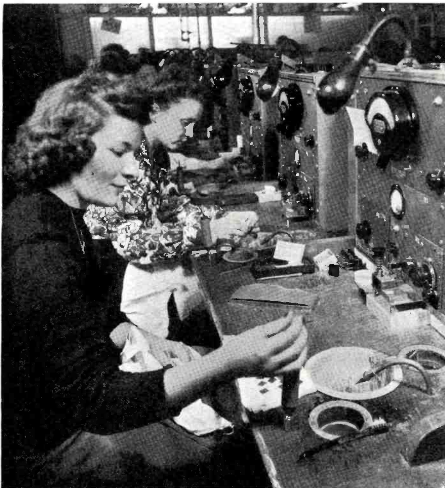
Crystals being etched to exact frequency prior to final assembly.
