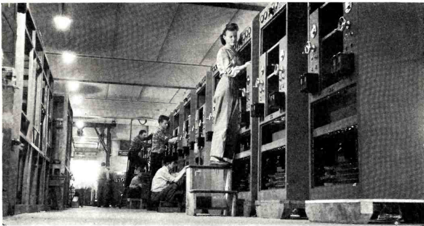
Mechanical assembly line of 2½-kw. transmitters at a Press Wireless plant. Note wooden skids.
