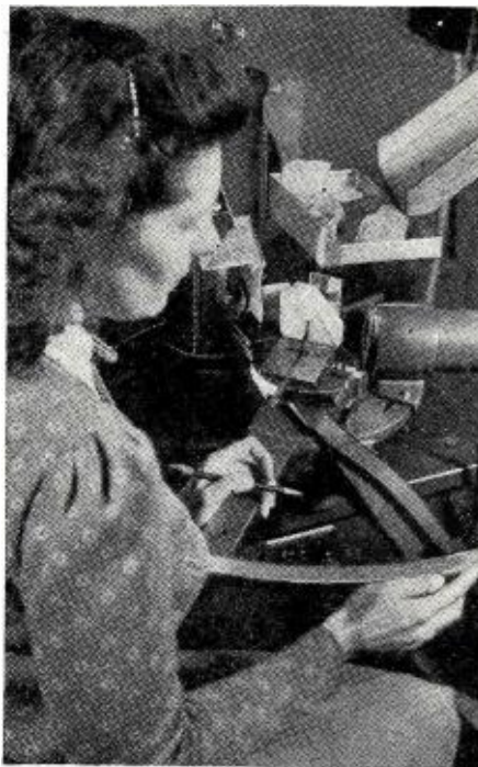
Taking X-ray measurements for angles of cut (angles from crystallographic axes) and direction.
