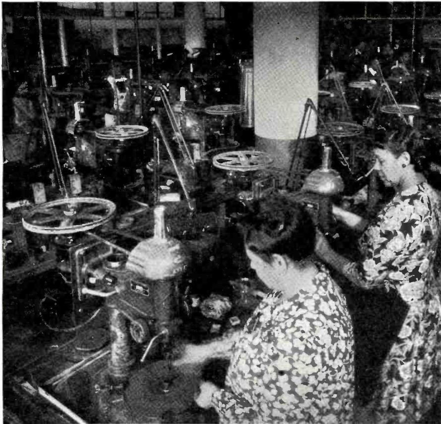
Automatically lapping, or grinding, crystals to approximate thickness.
