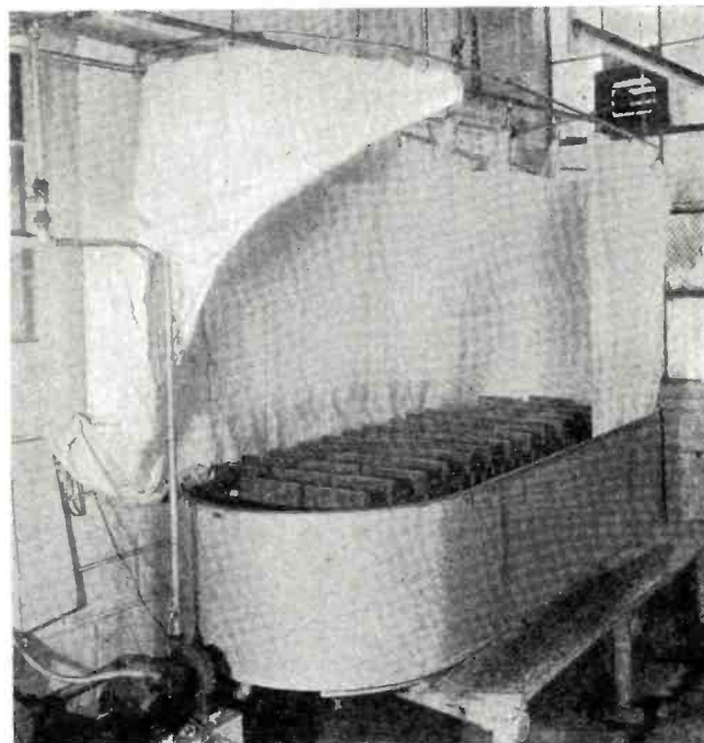
The tops of the walkie-talkie units are visible while undergoing the rain test. Overhead may be seen the jets from which water is sprayed during the required two-hour period. A certain percentage also receives a 24-hour rain test. This test is given in addition to a simple immersion test, which is made to reveal any imperfections or pinholes that may have resulted during assembly. After the test is made, the presence of four or five drops of water inside the case is considered sufficient for rejection. This is the final test and after its completion the walkie-talkie units are prepared for shipment to our Armed Forces.
