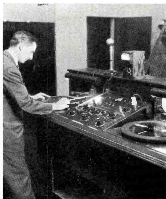
Closeup of dubbing table. Controls include automatic studio control board, filters, and equalizers.
