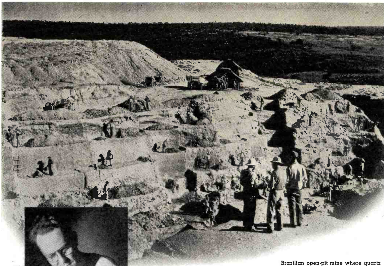
Brazilian open-pit mine where quartz is obtained entirely by hand labor.
