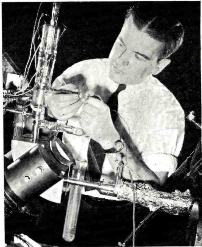
The key part of the mass spectrometer, a newly-designed electronic tube to be used in the gasoline and synthetic rubber industry. A magnet draws electrified molecules towards a target, where they are collected and their electrical charges counted by meters, enabling an accurate check of the composition of the mixture being tested.
