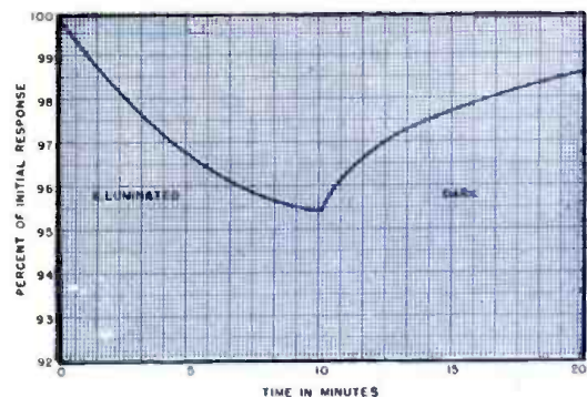
Fig. 9. Recovery curve of standard photocell from period of complete darkness to full illumination.
