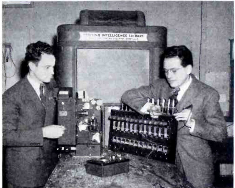
Fig. 1. The inventor, Mr. Morse (left), inspecting the projector and photocell-relay keying panel. In the rear can be seen the Panoram movie screen.
