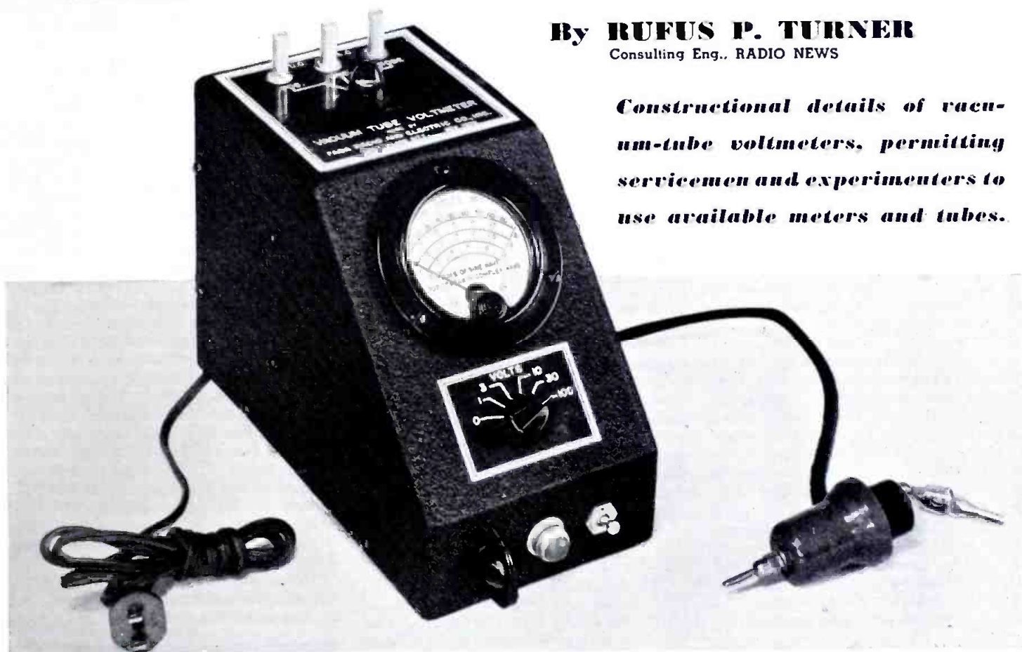
Vacuum-tube voltmeter described in the September, 1943 issue of RADIO NEWS. This instrument utilized a 0-200 microammeter. Circuits described herein will show how less sensitive meters can be substituted.
