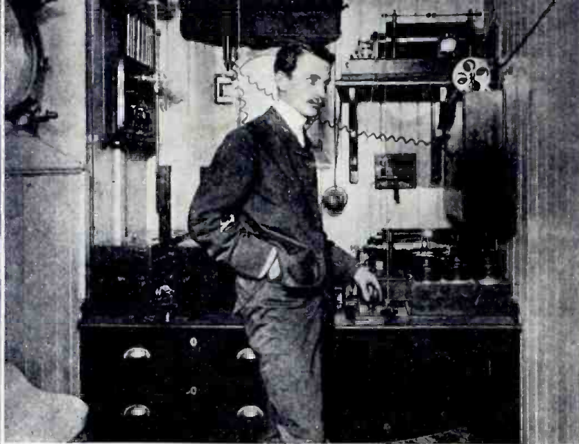
Early ship installation, British Marconi 1902 spark transmitter. (Left) shielded receiver and coherer; (right) open-type spark-gap.
