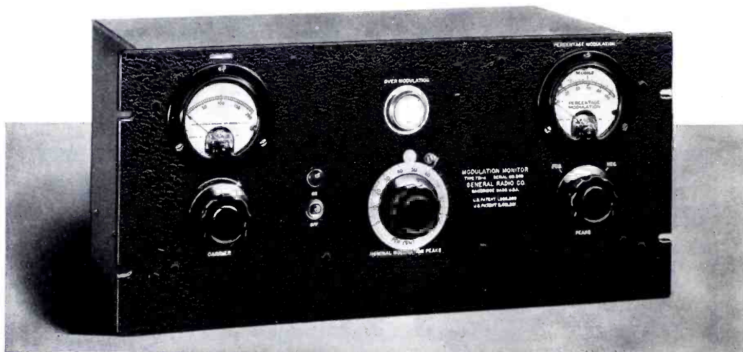
Fig. 1. Commercially constructed modulation monitor for checking modulation percentage of radio transmitters.
