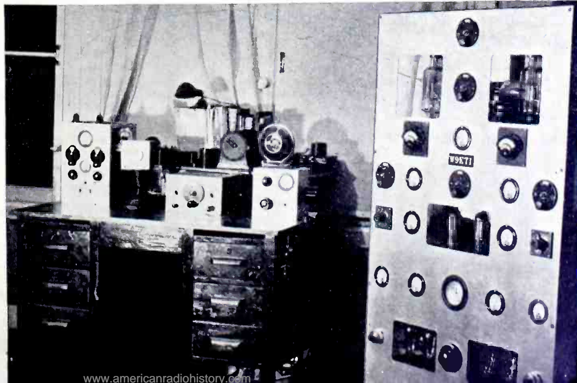
All-aluminum panels dressed the 1932 units. X'mtr had push-pull 400-w. screen-grid bottles, screen-modulated by 211-E's. Mike was double button carbon.
