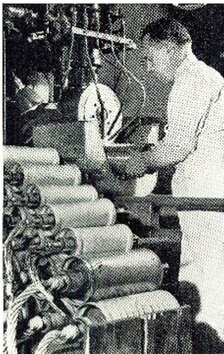
Ammunition for industry—the "ammunition being turned out by this workman are electronic tubes produced by the Westinghouse Lamp Division. Ignitrons, like these metal-encased devices, convert alternating current into direct current needed to make aluminum for American fighting planes. The workman is shown seam-welding the metal jacket in which tube mechanism is enclosed.
