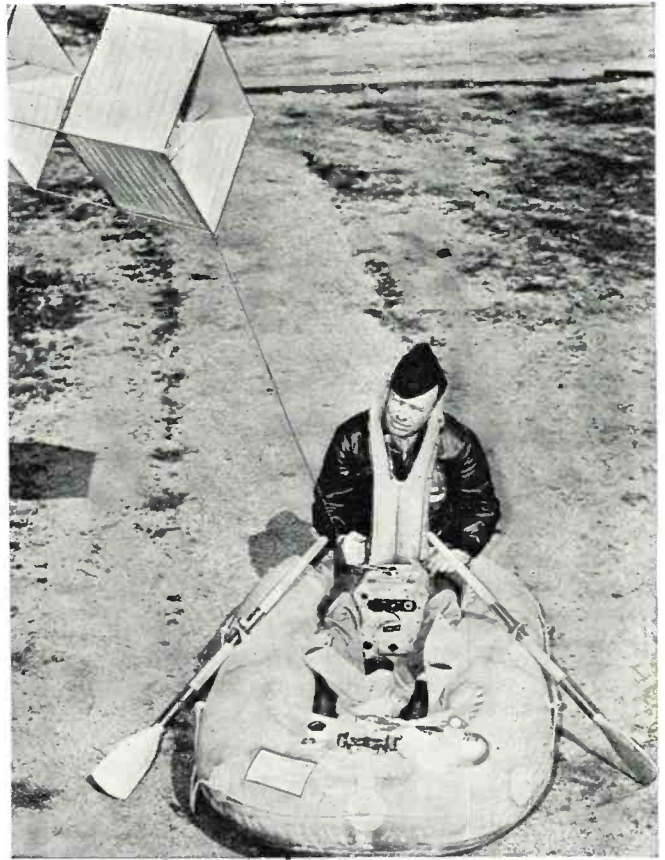
Life raft is equipped with kite antenna and automatic SOS transmitter which provides means of locating lost pilot.
