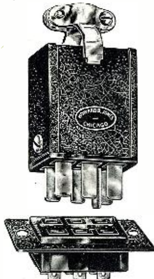
The socket contacts are of phosphor bronze, silver plated. The plug con-
