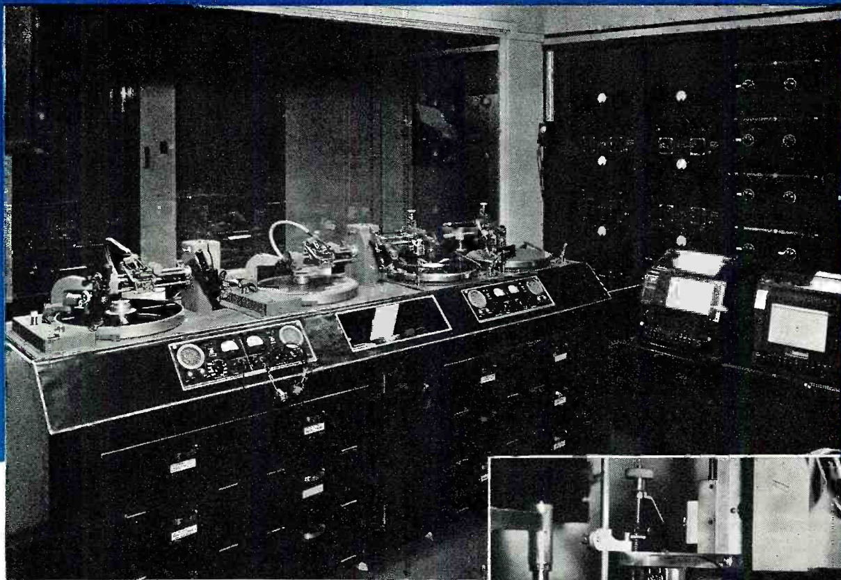
Recording equipment at station KOA, Denver—an example of a compact, smaller station type installation, consisting of four complete channels. (Insert) An RCA high fidelity cutter head during actual recording. Sapphire stylus can be seen bearing on record. Upright flanged tube to left is a suction nozzle used to remove chips from path of cutting stylus.
