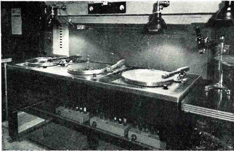
Portions of each of two or three recordings can be "taken off" to be combined as a single program on a new record.
