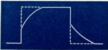
Fig. 11. Distortion of a square light pulse.
