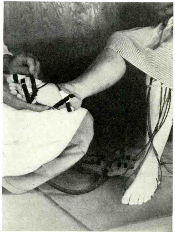
Pressure discs being applied to foot before recording walking-gait characteristics, with oscillograph using galvanometers.
