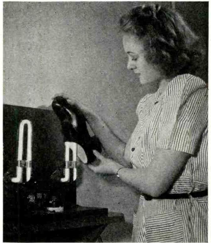
A horseshoe-shaped ultra-violet ray lamp used by a large industrial plant to prevent spreading of foot infections.
