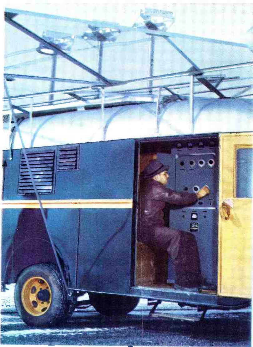
One of the most interesting pieces of equipment used by CAA engineers is this portable high-frequency localizer. It saves valuable testing time.
