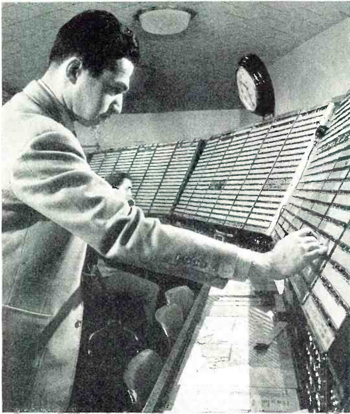
Airways Traffic Control Center. On each of these slots is recorded complete data of individual flights over Federal Airways.
