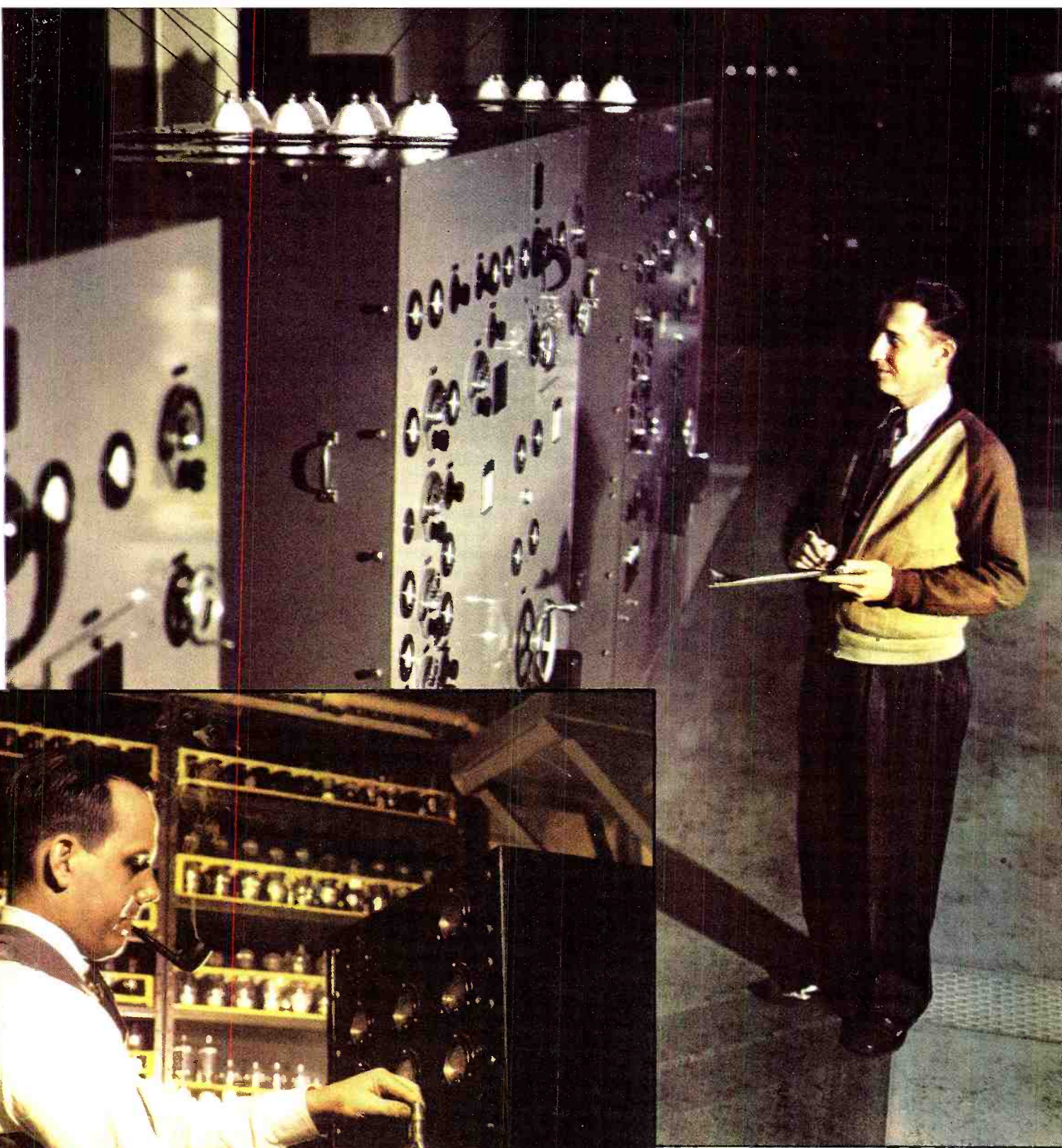
Specially-designed 20kw. transmitters at the CAA intercontinental radio station, Sayville, L. I., have world-wide coverage. Air-cooled tubes are used.
