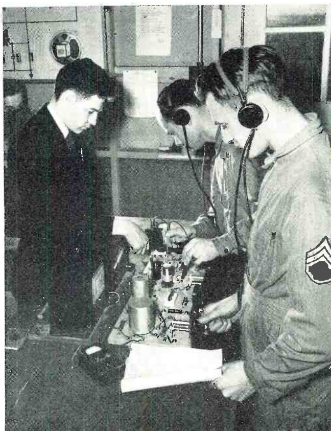
Breadboard-style transmitter undergoes a series of tests while instructor gives helpful suggestions to students.
