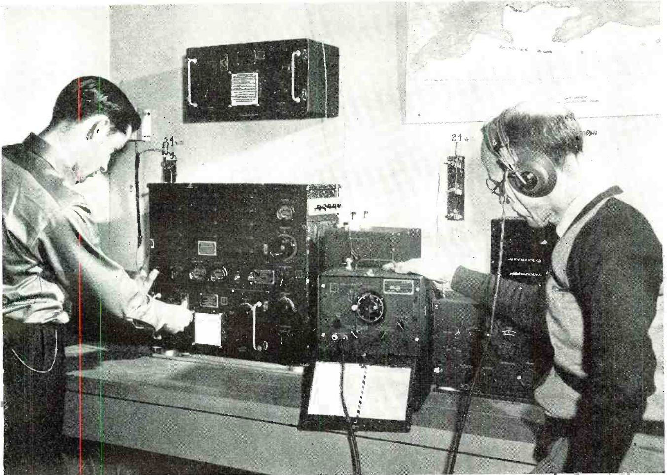
Maintenance men testing and realigning an aircraft communications receiver. Such equipment must be serviced periodically.
