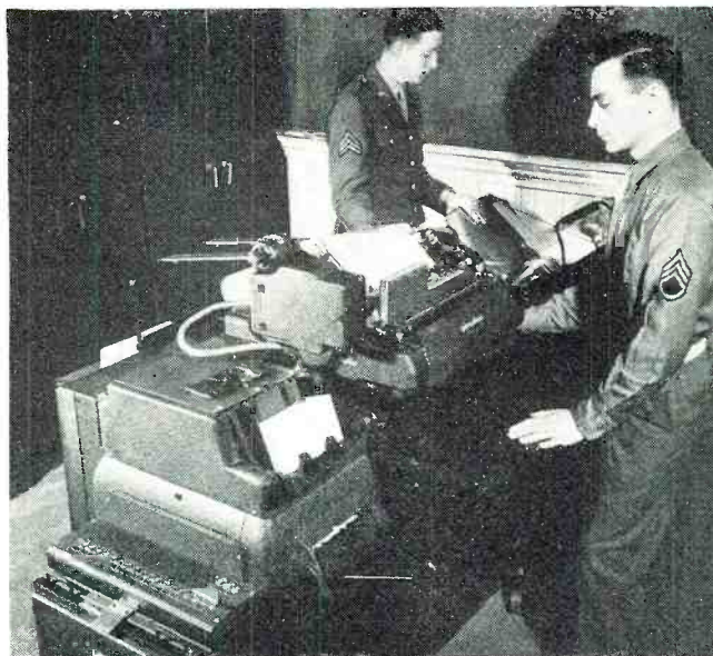
Tabulating and Accounting machine and Transfer Posting machine complete tabulation of code speeds and scholastic records of all kinds.
