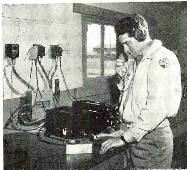
Radio set for aircraft undergoing an operational test before being installed permanently within military plane.
