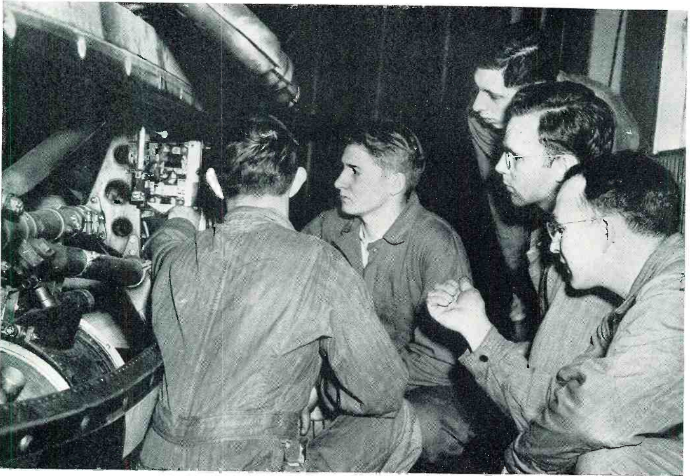
Instructor explains voltage control and regulator unit on a P-40 pursuit ship to students.
