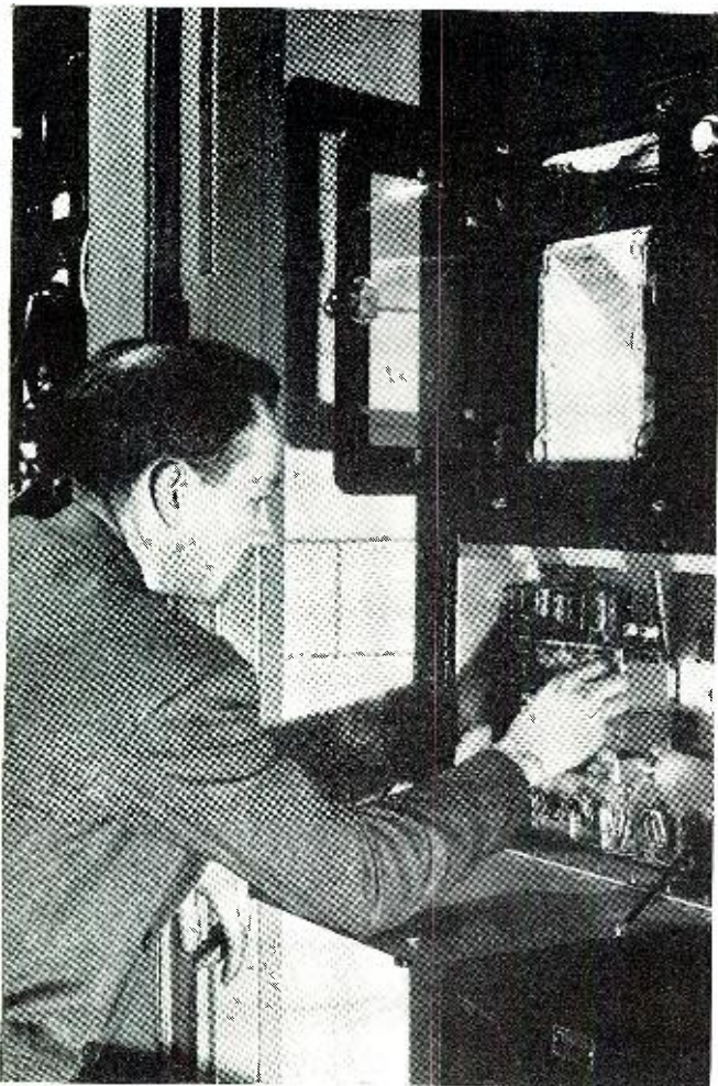
Fig. 9. Operator making adjustment on the instrument landing system control rack. Elaborate equipment is necessary.
