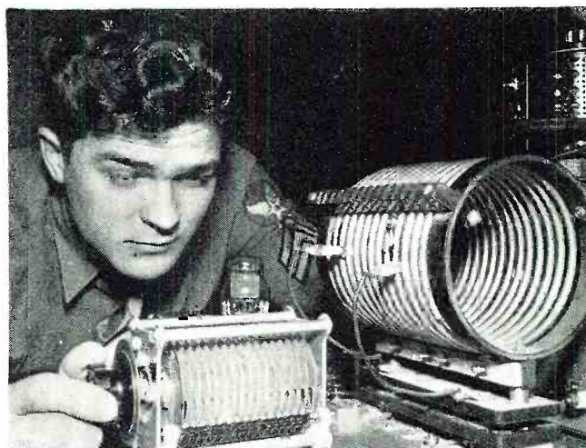
Student brings tank tuning condenser to resonance with the large transmitter RF tank coil. Clips permit proper L/C ratio for best output.
