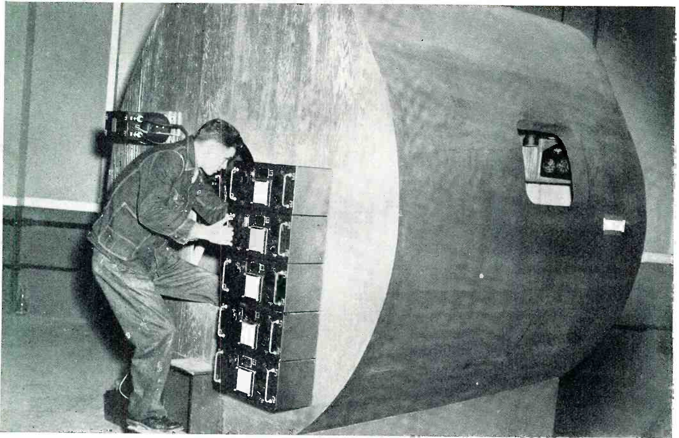
Operator entering a completely radio equipped mock-up of a B-26 bomber. Transmitter tuning units are in foreground.
