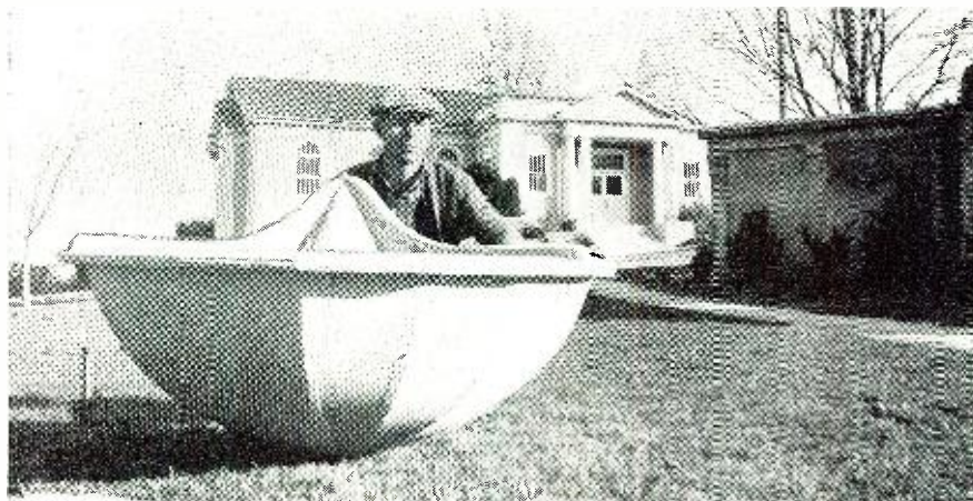
Showing relative position of pickup speaker as it would appear when in actual airplane detecting.
