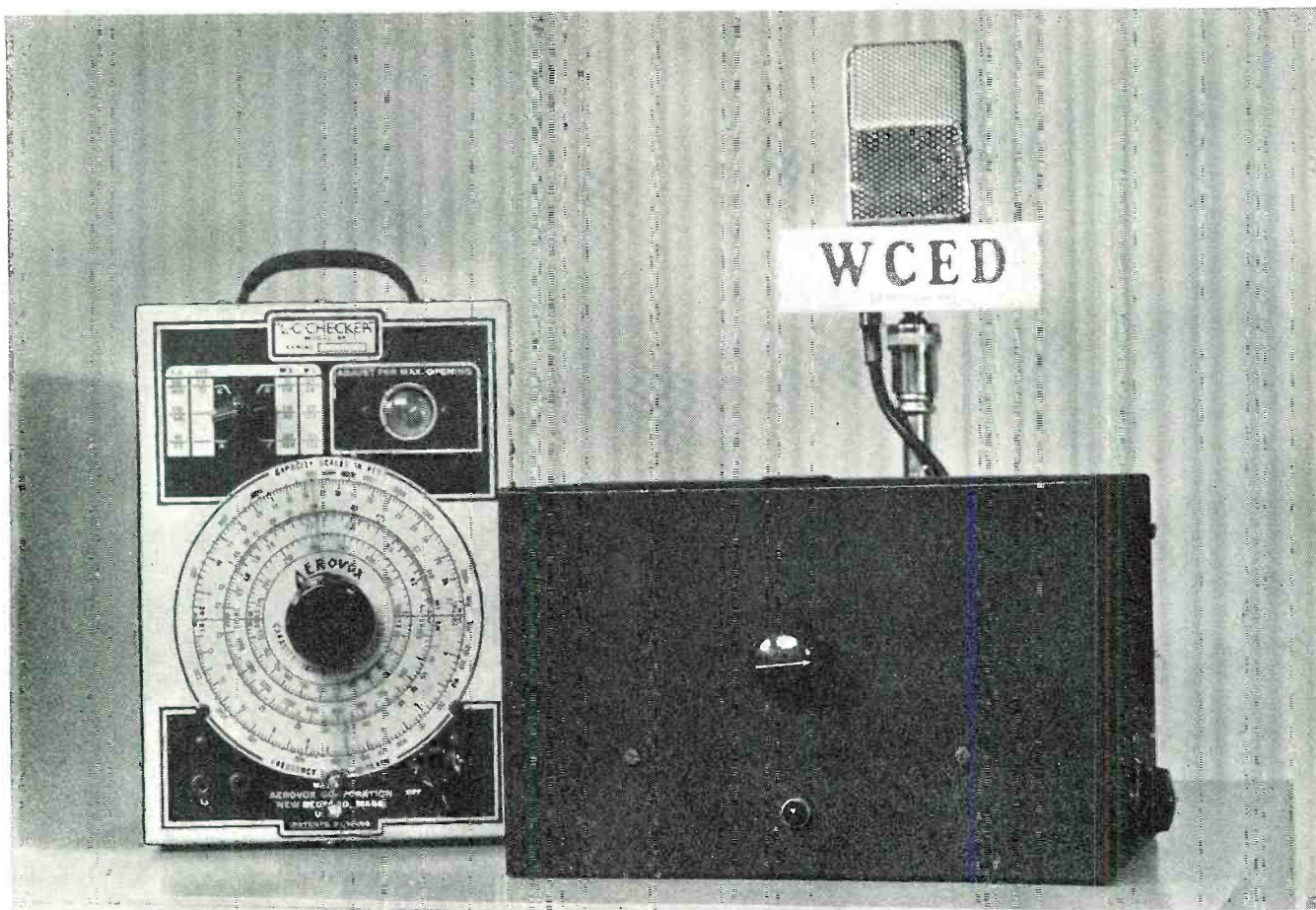
Knob for pitch adjustment is in panel center—Regeneration control on side.
