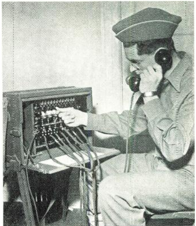
Orders are sent over this portable switchboard to direction-finders in the field to locate enemy.
