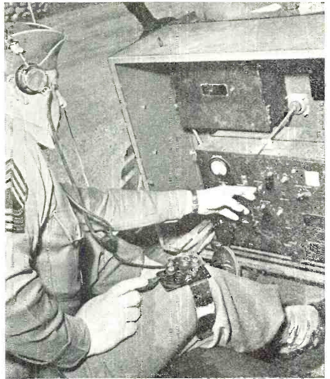
Non-commissioned officer in command car talks with intercept headquarters. Note key on his leg.
