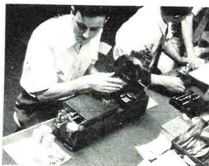
Checking gears for condenser to be used on aircraft radio equipment.
