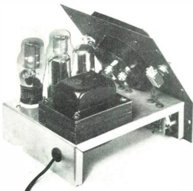
Easier reading of the meter is afforded by using a metal cabinet that is constructed with the panel at an angle. Panel mounts last.
