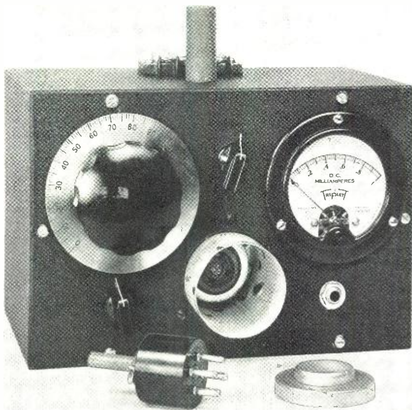
Coils plug in the shield can. Basic instrument is a 0-1 DC milliammeter.
