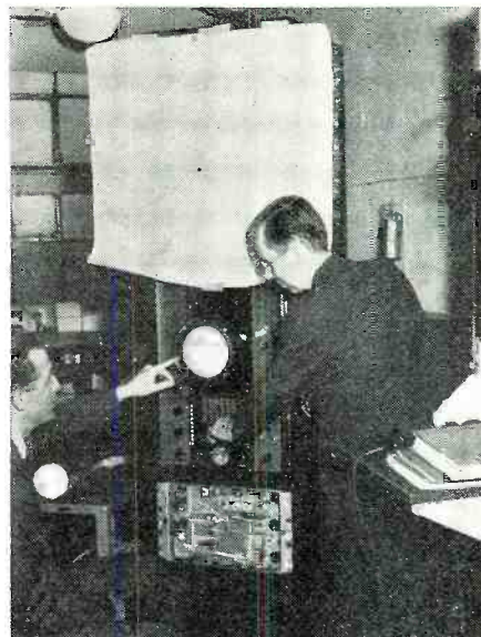
Fig. 6. Azimuth indicator located at one of our large eastern airports.
