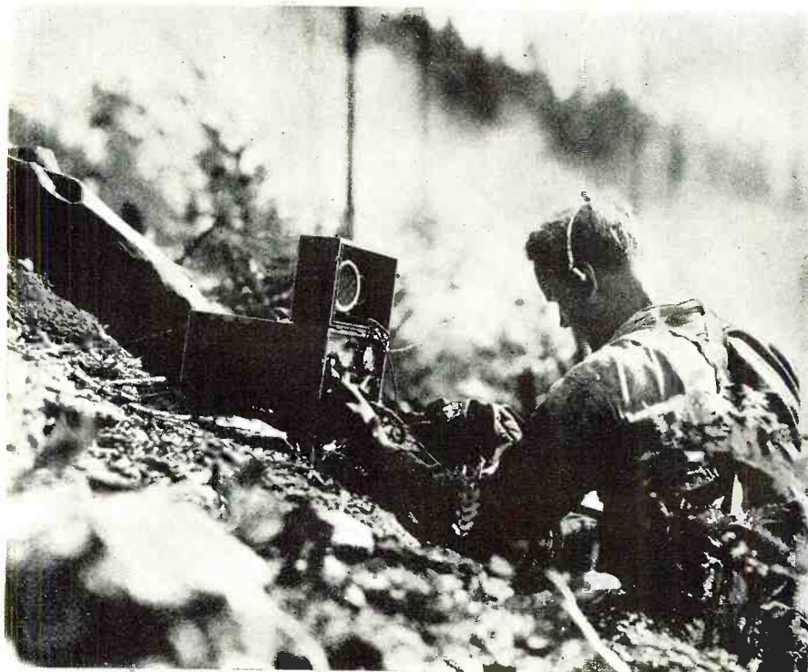
Emergency radio station, fire line, Spud Hill fire. Note featherweight phones.
