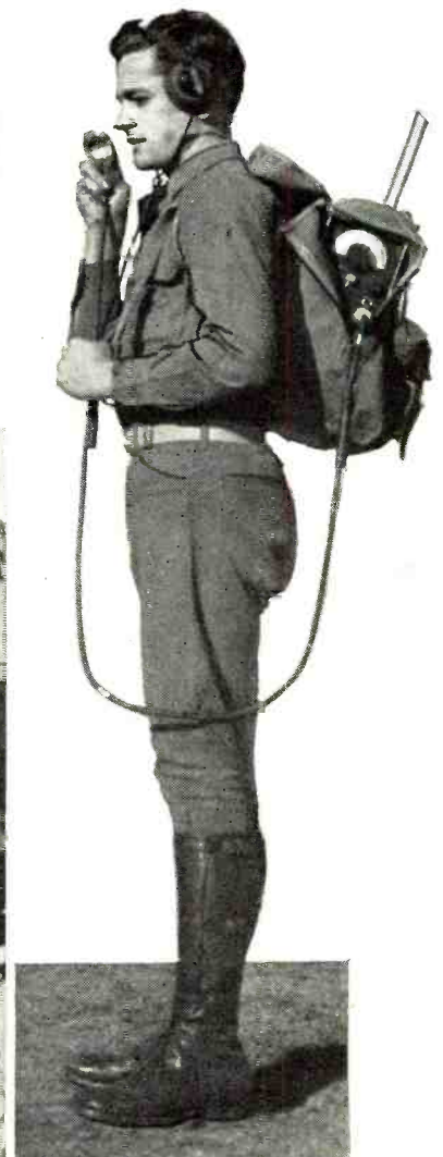
Right: SCR-194 Walkie-Talkie used at observation post to communicate with gun positions uses phone only.
