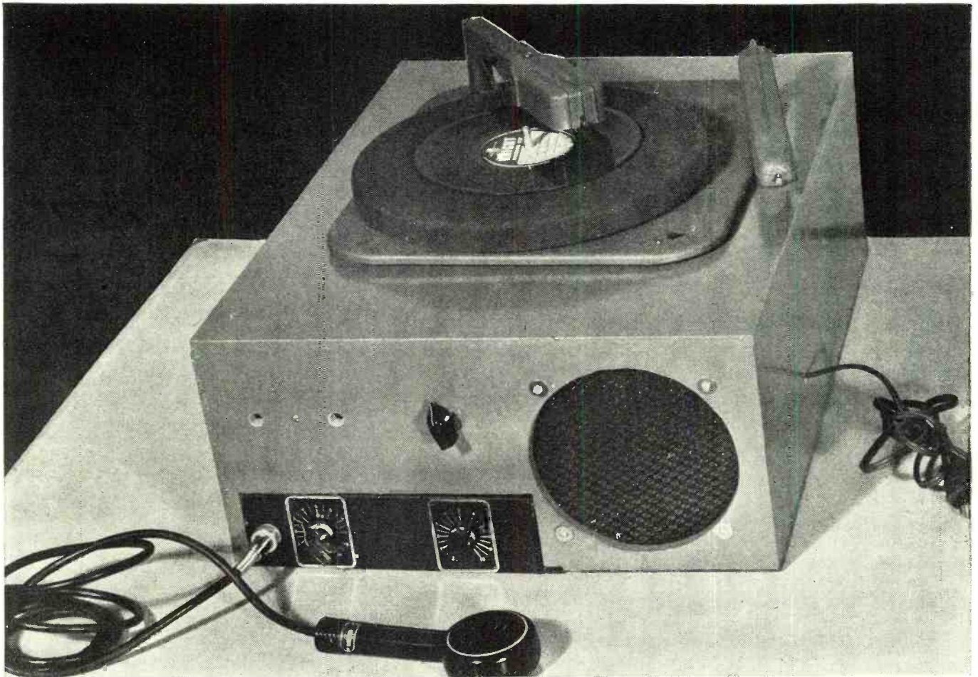
An inexpensive diaphragm-type crystal microphone gives satisfactory results with this recorder.
