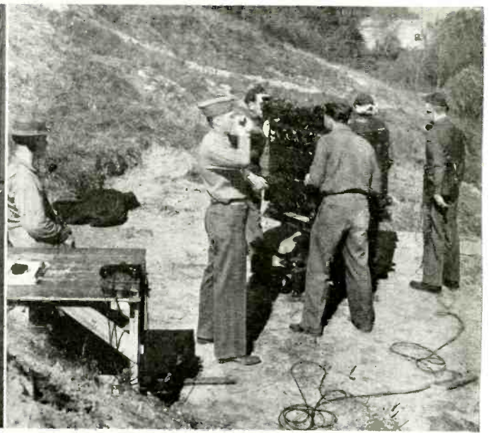
Anti-aircraft gun data-computer at Fort Sheridan which is connected to the guns by cable. Note telephone sets.
