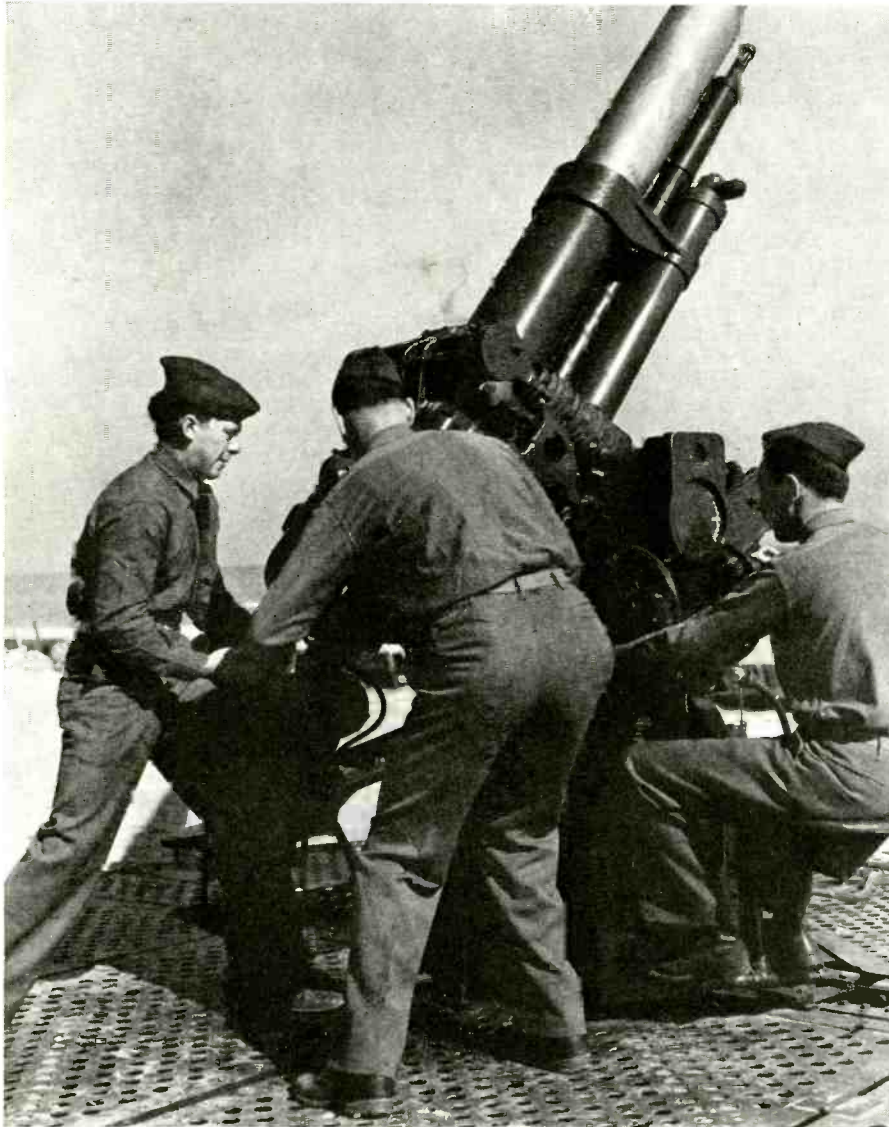
The business end of the setup. The operator is seated facing an indicator dial. When two arrows match it shows that the gun is "on the target."
