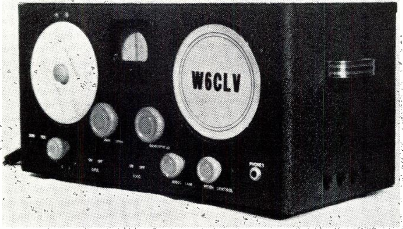
The converted set takes on a most pleasing appearance. The escutcheon is cut from cardboard.
