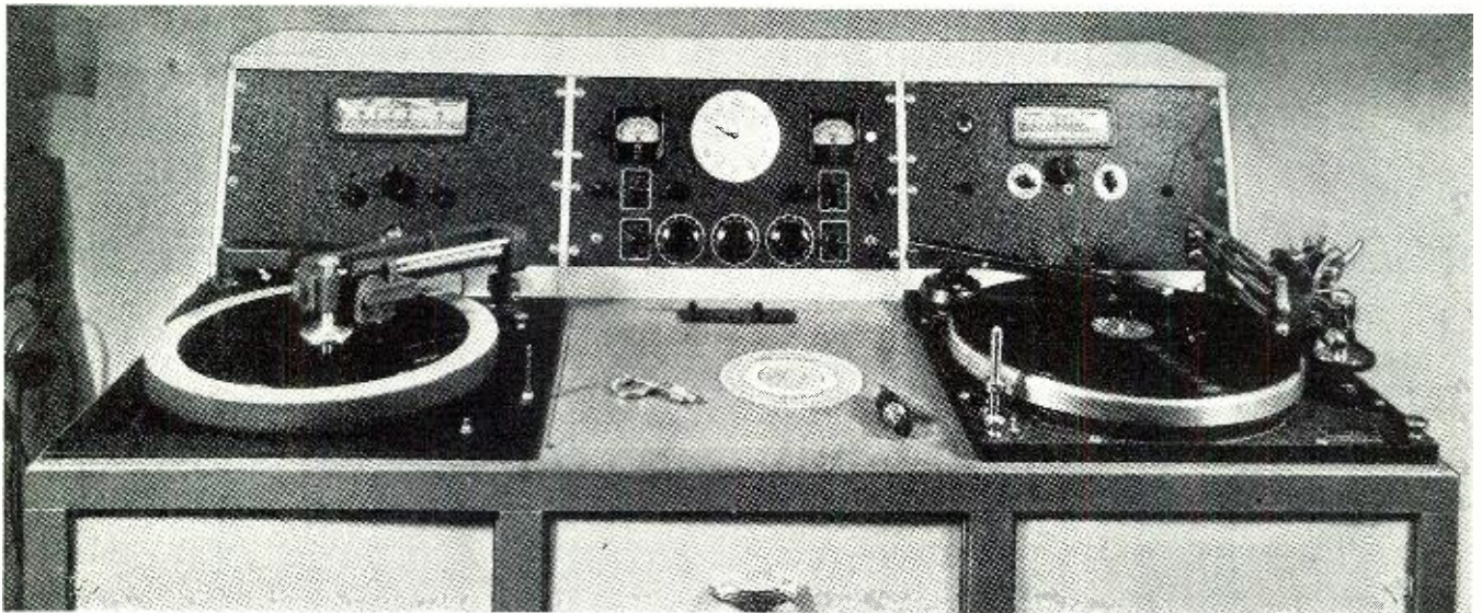
The author's recording console designed for flexibility and ease of operation. Continuous recording requires two tables.
