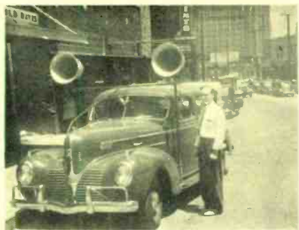
The method used to mount the speakers is clearly shown in these two illustrations. Note all the bracing.
