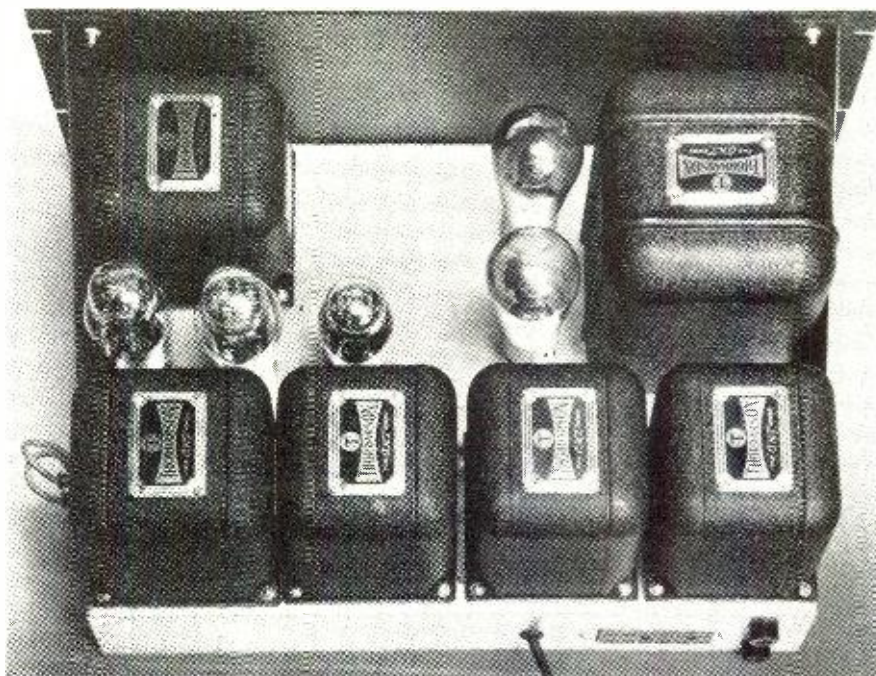
The 800-volt power supply chassis. The layout is smaller for 2A3's.
