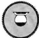
Only edges of shaft are filed for odd types.
