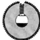
How shaft is positioned for set-screw knob.
