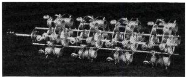
The laboratory-built band-change switch which contains all the AM antenna and R.F. coils. Pies are self-shorting type of isolantite.
