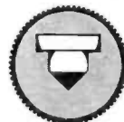
Shaft position in knob requiring 1/32" flat.
