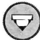
Shaft position in knob requiring 3/32" flat.
