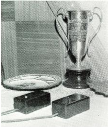
Buzzer transmitter and receiver; signal for children or invalids.
