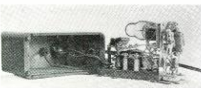
Inside detail of the OA4G receiver. Note the very rugged construction.
