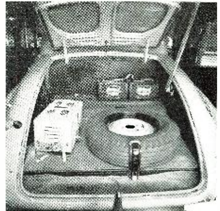
The trunk installation. Two storage batteries power the final amplifier. The final is to the left next to the tire, and is controlled by cables.
