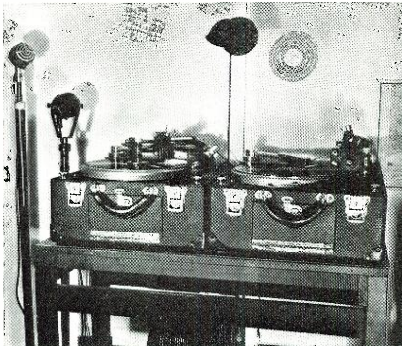
Continuous recordings require that two turn-tables be used.
