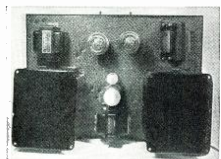
Top view of the power supply chassis.
