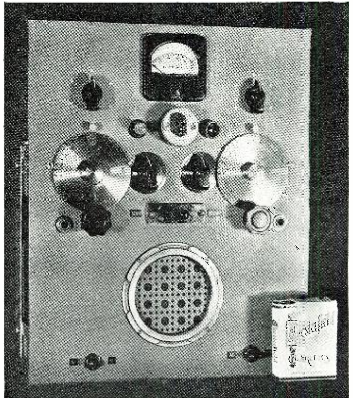
Compact, the rig works from 6v.dc or 110v.ac power.
