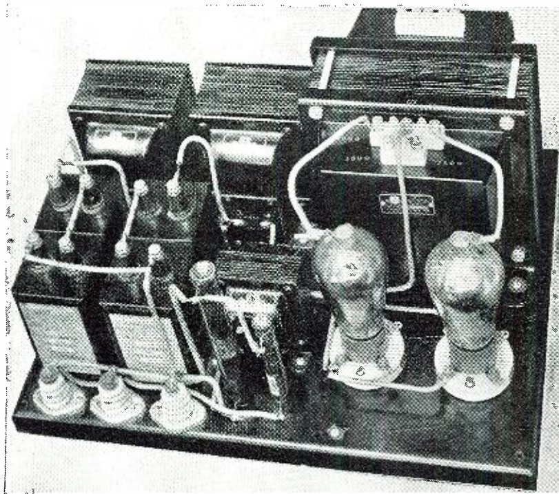
In building this power supply the leads were all kept above the chassis for greater safety and for servicing.
