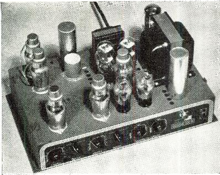
Notice the ventilation holes for the resistors underneath.
